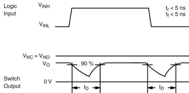
Figure 2. Break-Before-Make Interval
