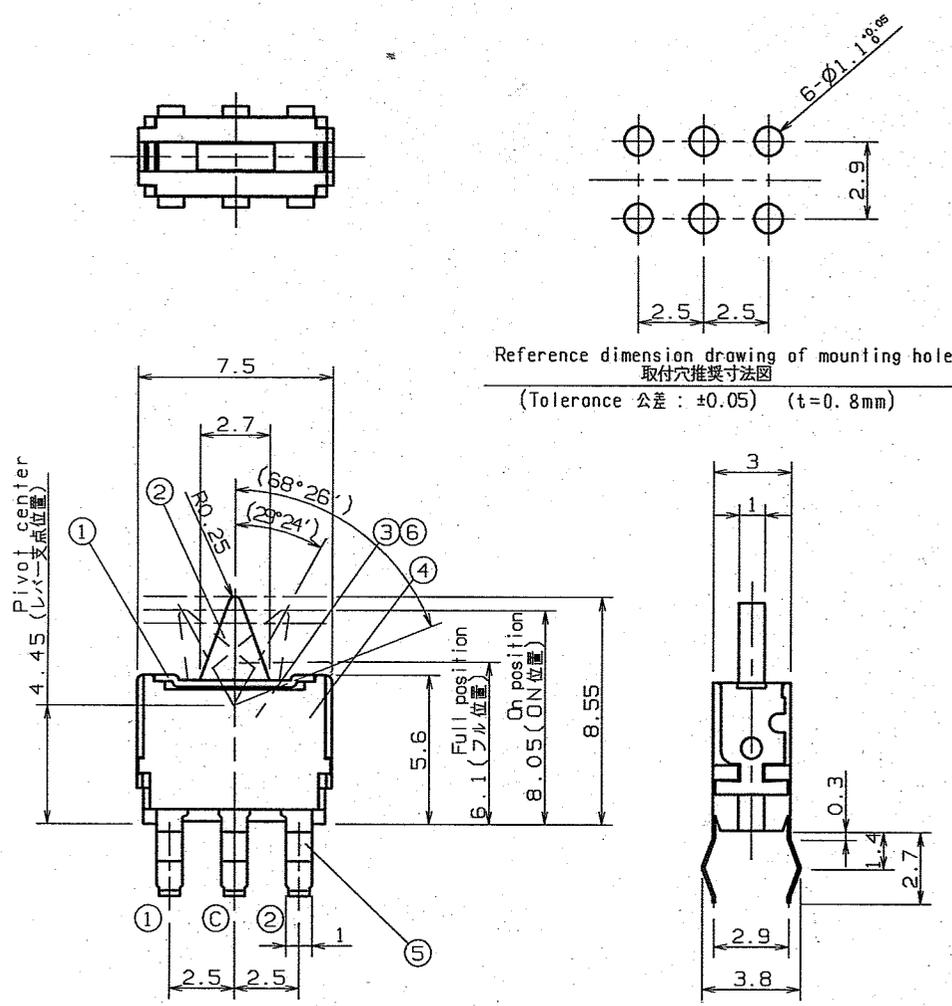
Reference dimension drawing of mounting hole
