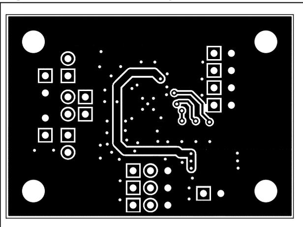
Figure 9. Top view of the demonstration board
