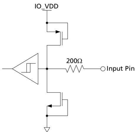
Figure 3-3: Digital Input Pin with Schmitt Trigger (RESET)
