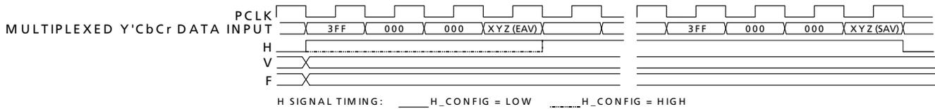
**Figure 4-5: H:V:F Input Timing - SD 10-bit Mode**
