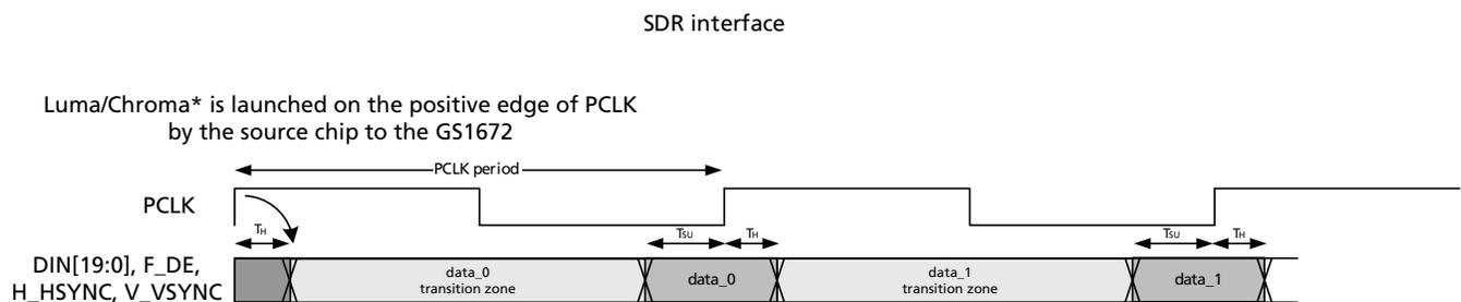
Figure 4-1: GS1672 Video Host Interface Timing Diagrams
