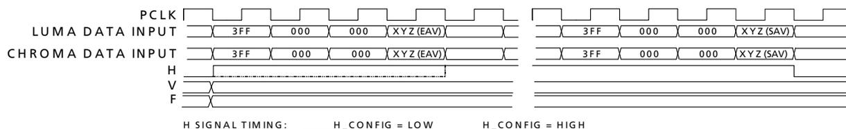
Figure 4-2: H:V:F Input Timing - HD 20-bit Input Mode
