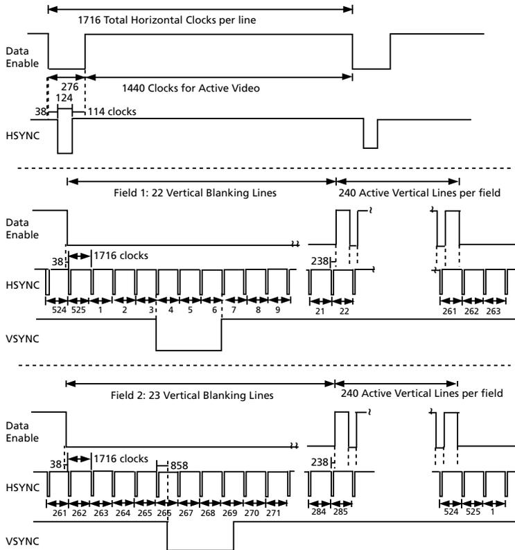
**Figure 4-8: H:V:DE Input Timing 720 (1440) x 480i @ 59.94/60 (Format 6&7)**
