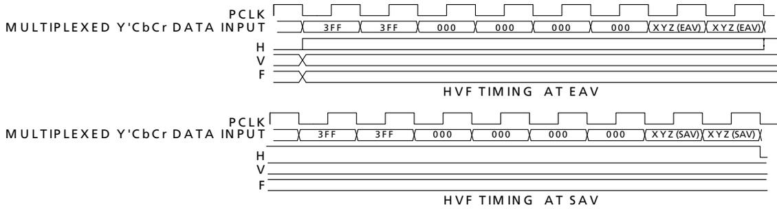
**Figure 4-3: H:V:F Input Timing - HD 10-bit Input Mode**
