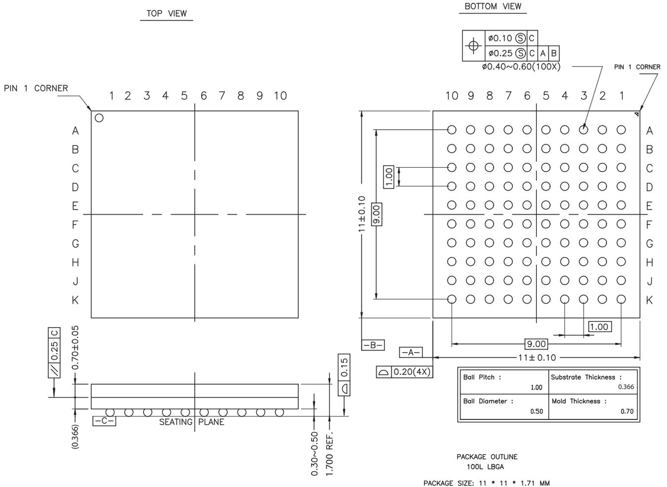
\* THE BALL DIAMETER, BALL PITCH, STAND-OFF & PACKAGE THICKNESS ARE DIFFERENT FROM JEDEC SPEC M0192 (LOW PROFILE BGA FAMILY)
