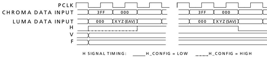
**Figure 4-4: H:V:F Input Timing - SD 20-bit Mode**
