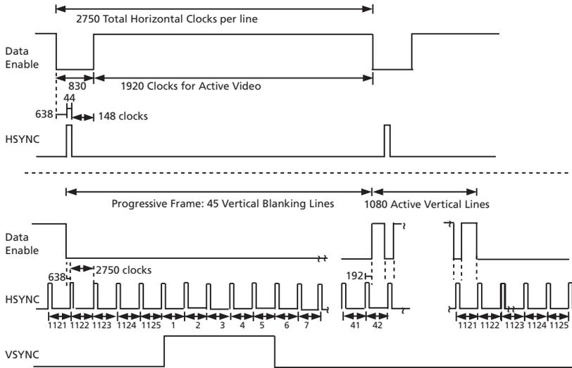
**Figure 4-12: H:V:DE Input Timing 1920 x 1080p @ 23.94/24 (Format 32)**
