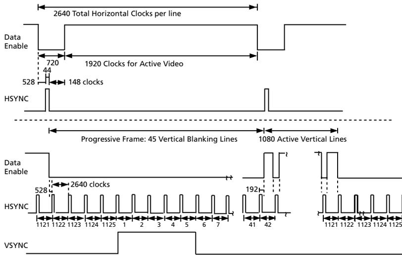
**Figure 4-13: H:V:DE Input Timing 1920 x 1080p @ 25 (Format 33)**
