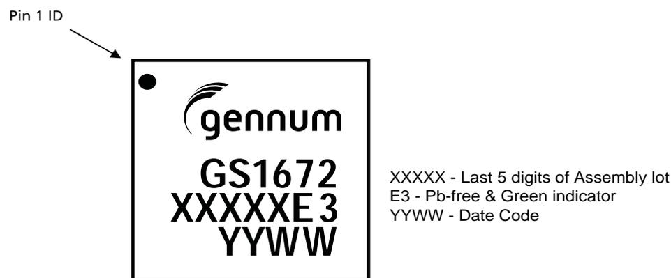
**Figure 7-2: Marking Diagram**
