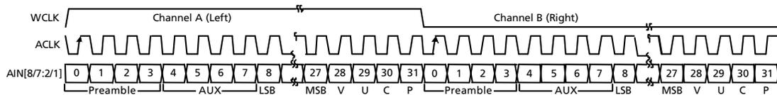
**Figure 4-17: AES/EBU Audio Input Format**
