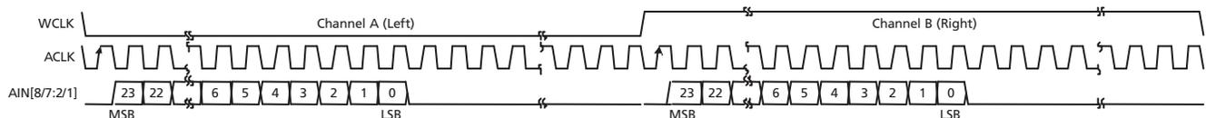
**Figure 4-16: I<sup>2</sup>S Audio Input Format**
