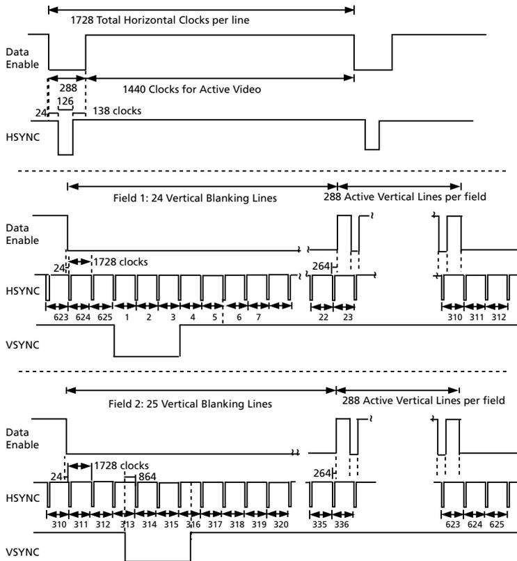
**Figure 4-11: H:V:DE Input Timing 720 (1440) x 576 @ 50 (Format 21&22)**
