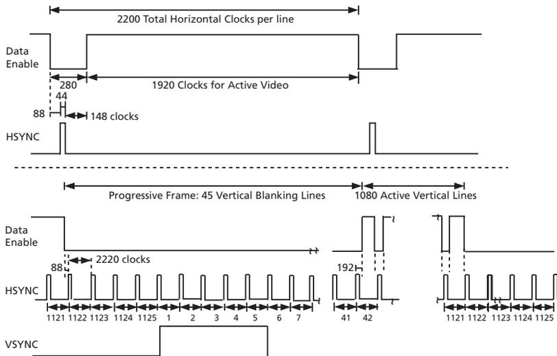
**Figure 4-14: H:V:DE Input Timing 1920 x 1080p @ 29.97/30 (Format 34)**
