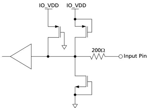
**Figure 3-5: Digital Input Pin with weak pull-up - maximum pull-up current <math>< 110\mu\text{A}</math> (ACLK1, ACLK2, AIN\_7/8, AIN\_5/6, AIN\_3/4, AIN\_1/2, CS\_TMS, GRP1\_EN/DIS, GRP2\_EN/DIS, IOPROC\_EN/DIS, SDO\_EN/DIS, TMS, WCLK1, WCLK2)**
