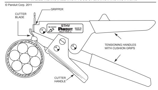
**NOTE:** This precision tool has been engineered and designed for use with Panduit nylon cable ties up to .35" wide. It is not intended for other uses such as cutting or tensioning wires or other types of fastening devices.
