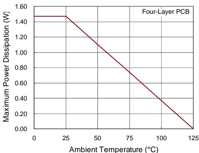
Figure 8. Derating Curve for RT8510 Package
