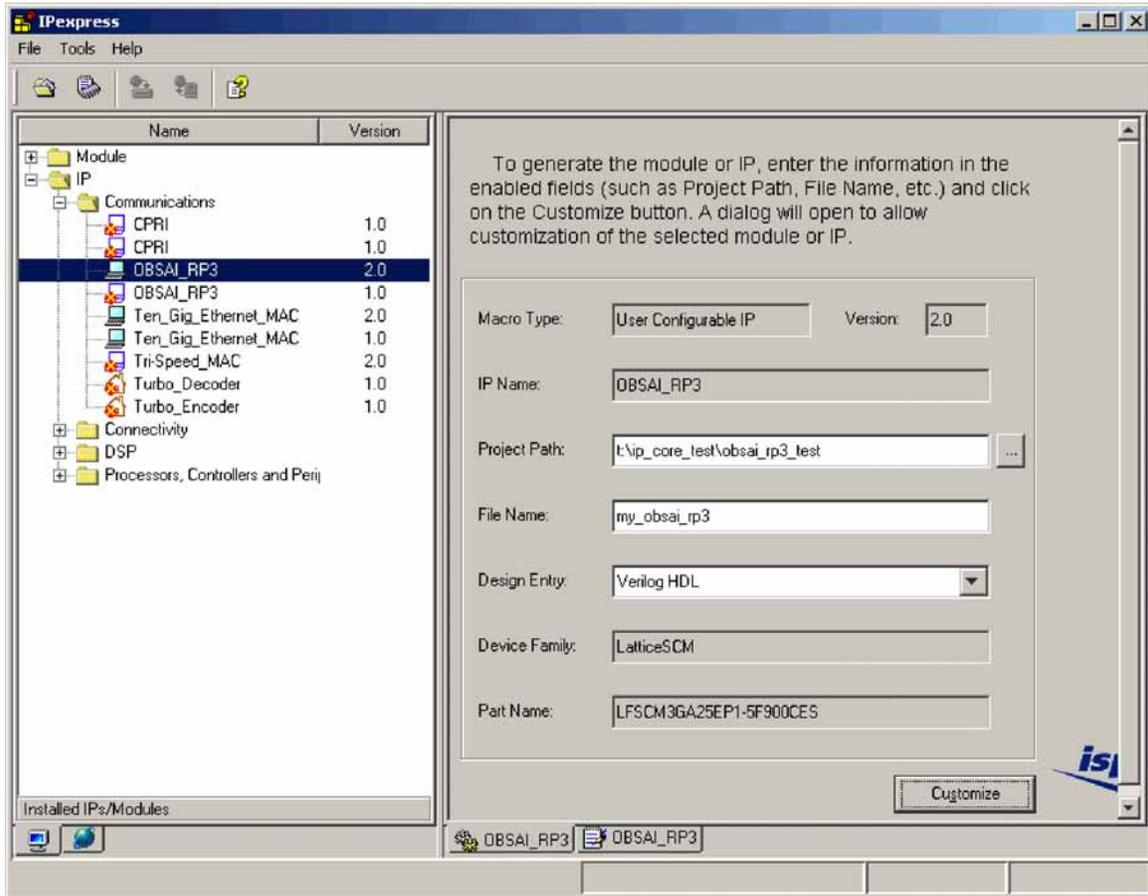
To create a custom configuration, click on the **Customize** button to display the OBSAI RP3 IP core Configuration GUI, shown in Figure 11. From this window, the user may select the desired OBSAI RP3 configuration parameters.
