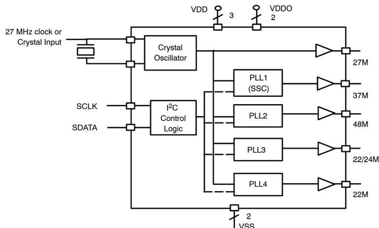
Figure 1. Block Diagram
