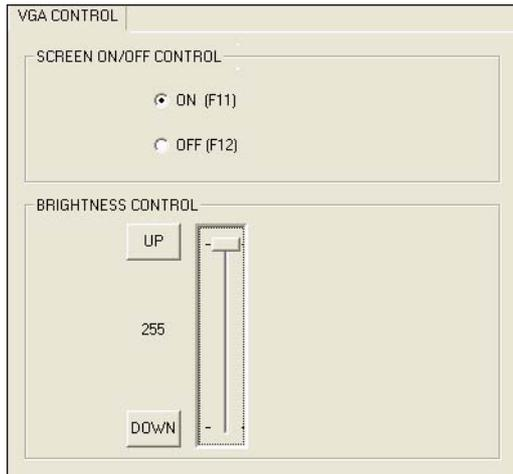
When the application is executed, it will display two blocks of VGA control functions. The application can turn on or turn off the screen shot freely, and it also can tune the brightness of the panels if your platform is being supported. You can test the functionalities of VGA control as follows:
