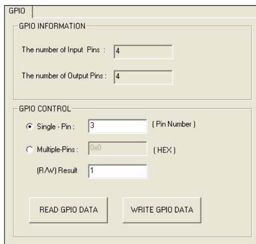
When the application is executed, it will display GPIO information in the GPIO INFORMATION group box. It displays the number of input pins and output pins. You can click the radio button to choose to test either the single pin function or multiple pin functions. The GPIO pin assignments of the supported platforms are located in Appendix B.
