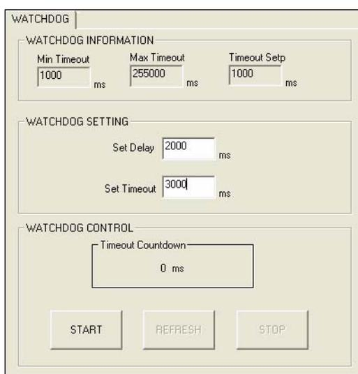
When the application is executed, it will display watchdog information in the WATCHDOG INFORMATION group box. It displays max timeout, min timeout, and timeout steps in milliseconds. For example, a 1~255 seconds watchdog will have 255000 max timeout, 1000 min timeout, and 1000 timeout steps. You can test the functionality of the watchdog as follows:
