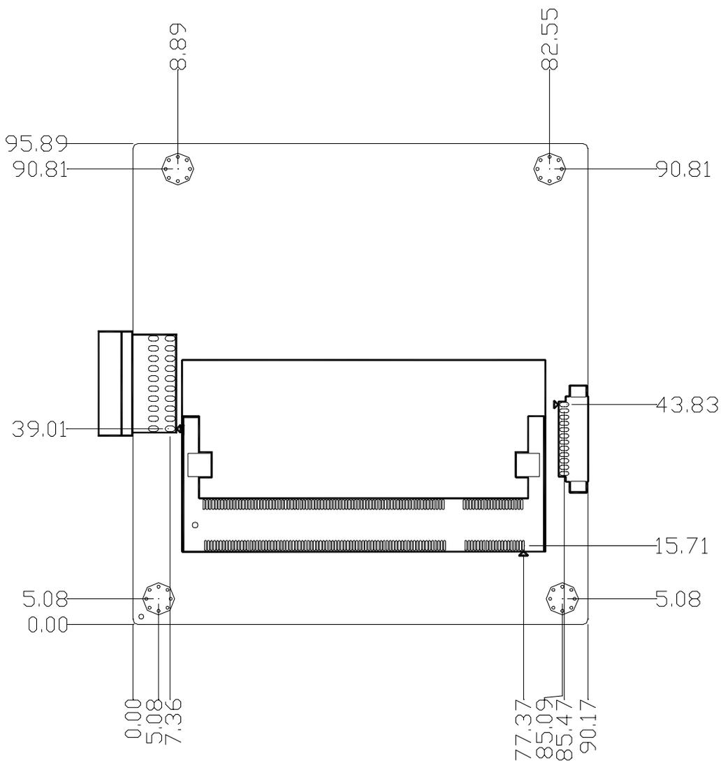
Figure C.2 PCM-3362 Mechanical Drawing (Solder Side)
