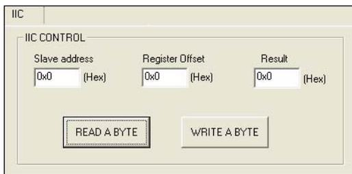
When the application is executed, you can read or write a byte of data through I2C devices. All data must be read or written in hexadecimal system.
