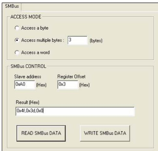
When the application has executed, you can click the radio button to choose to test each access mode, i.e. Access a byte, Access multiple bytes and Access a word. All data must be read or written in hexadecimal except the numbers for radio button: Access multiple bytes mode must be written in decimal. You can test the functionalities of the watchdog as follows:
