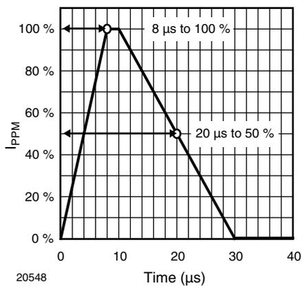
Fig. 2 - 8/20  $\mu\text{s}$  Peak Pulse Current Wave Form
