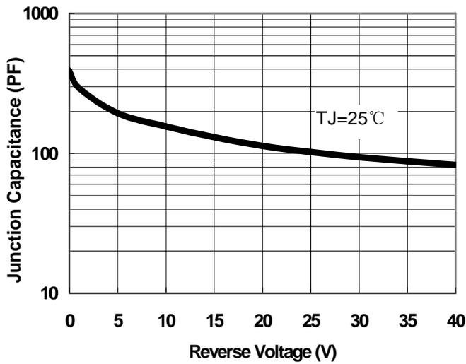
Fig.1-Typical Junction Capacitance
