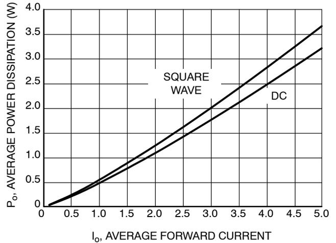
Figure 6. Power Dissipation
