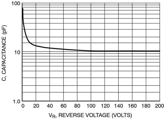
Figure 5. Typical Capacitance
