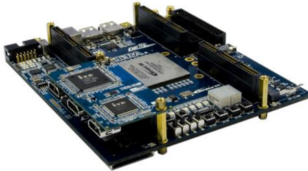
Figure 1-2 Connect HDMI daughter board to DE3 board
