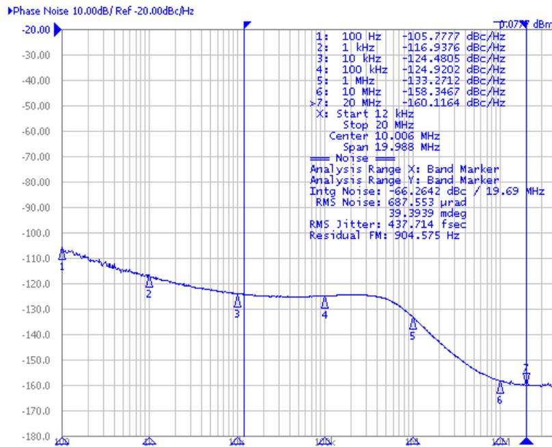
Figure 4. Typical Phase Noise Plot at 212.5 MHz
