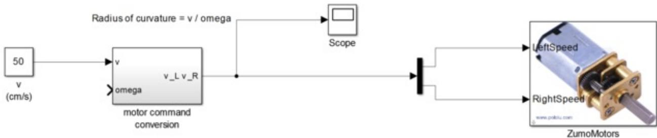
Thus with this workflow, at every time instant, we compute the position of the Zumo Robot relative to the black line. From that computation, we decide the amount by which the Zumo Robot should turn to continue staying on the line, and using that value we turn the Zumo Robot at that instant.
