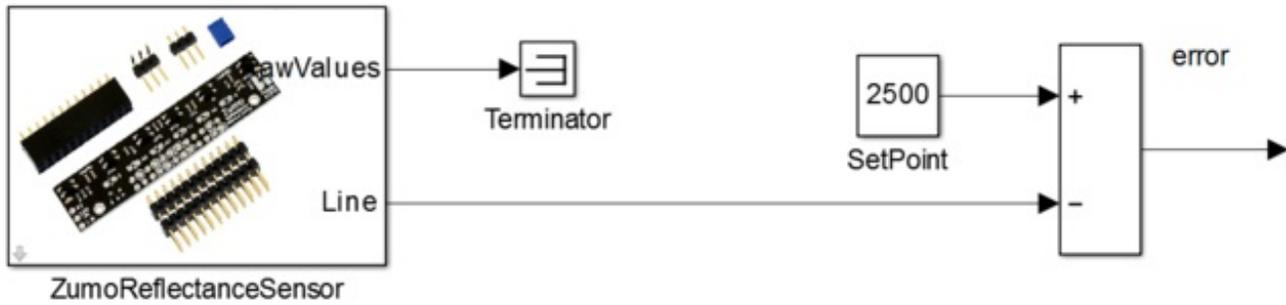
In the above block diagram, the '**ZumoReflectanceSensor**' block returns a numeric value as output. We then subtract 2500 from the numeric value to obtain the error signal which is then pushed further to the controller block. We will discuss the controller block on the next page.
