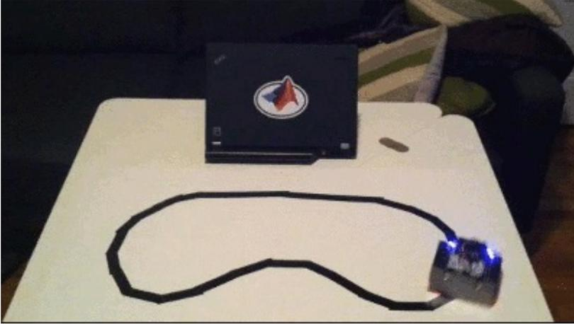
This tutorial covers how to use Simulink to program a Zumo Robot powered by an Arduino Uno to follow a line using the reflectance sensors present at the bottom of the Zumo Robot. This guide will explain how the data from the reflectance sensors can be used to control the Zumo Robot motors using a control logic known as PID control.
