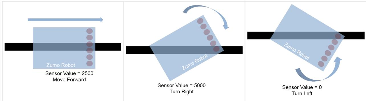
The simplest controller is illustrated in the figures above. The logic being: if the Zumo Robot center is to the left of the black line, then turn right by a fixed amount so that it eventually returns to the black line. Similarly, if the Zumo Robot center is to the right of the black line, turn left so that it returns to the black line. This controller is known as the Bang Bang Controller.
