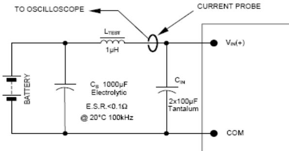
NOTE: Measure input reflected ripple current with a simulated source inductance ( $L_{TEST}$ ) of 1µH. Capacitor  $C_B$  offsets possible battery impedance. Measure current as shown above.
