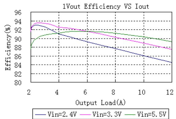
Figure 2: Converter efficiency vs. output current (1.0V out)
