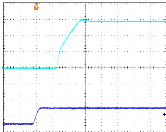
**Figure 11:** Turn on delay time at 5Vin, 0.6V/12A out(2mS/div), Top trace: Vout 0.2V/div; bottom trace: Vin, 5V/div
