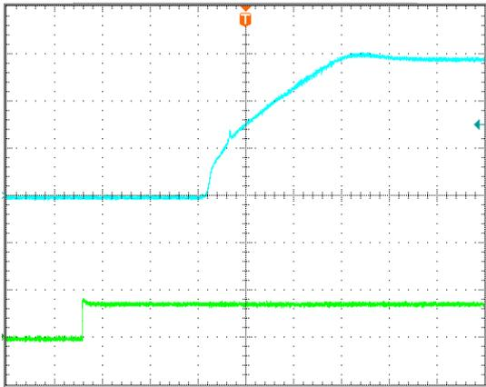
**Figure 15:** Turn on delay time at remote on/off, 0.6V/12A out(1mS/div), Top trace:Vout 0.2V/div; bottom trace: on/off,2V/div
