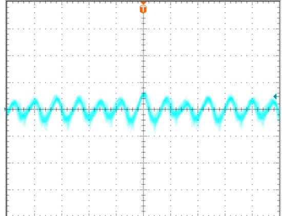
**Figure 8:** Output ripple & noise at 5Vin, 1.2V/12A out.
