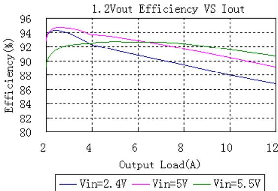
Figure 3: Converter efficiency vs. output current (1.2V out)
