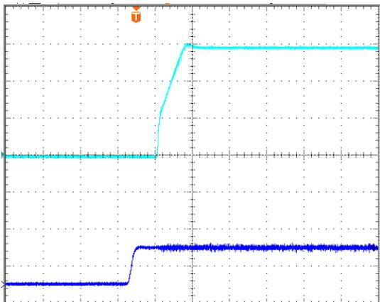
**Figure 17:** Turn on delay time at remote turn on with external capacitors ( $C_o = 800 \mu F$ ) 5Vin, 0.6V/12A out(4mS/div), Top trace:Vout 0.2V/div; bottom trace:Vin,5V/div
