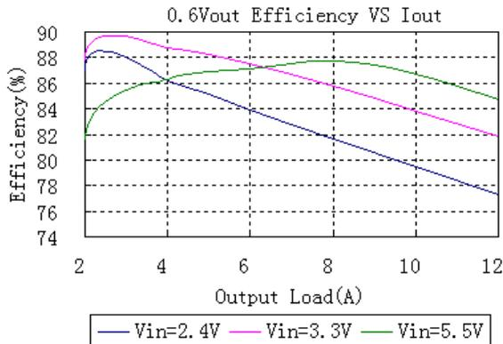
Figure 1: Converter efficiency vs. output current (0.6V out)
