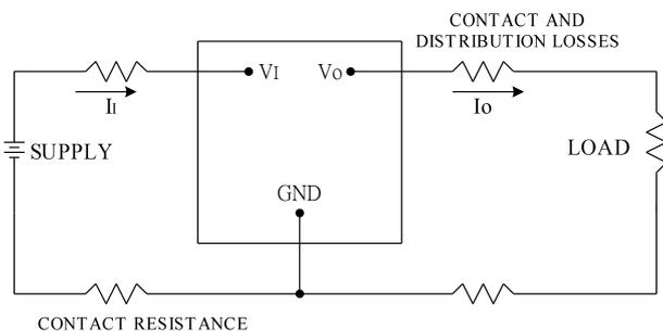
Figure 27: Output voltage and efficiency measurement test setup
