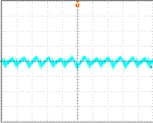
**Figure 7:** Output ripple & noise at 5Vin, 0.6V/12A out.
