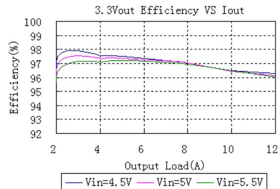
Figure 6: Converter efficiency vs. output current (3.3V out)
