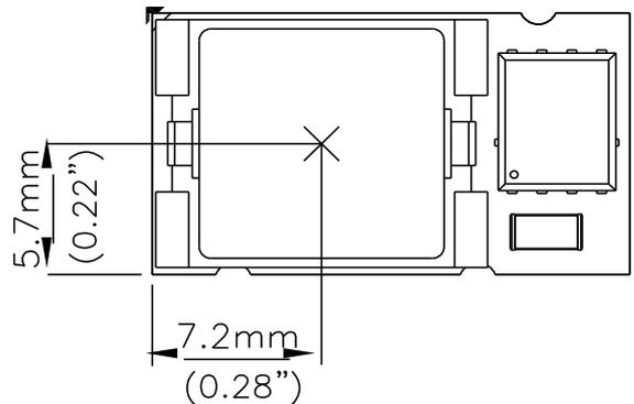
Figure 37: Temperature measurement location
