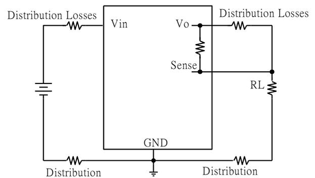
**Figure 30:** Effective circuit configuration for remote sense operation
