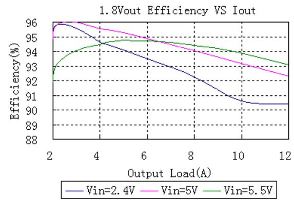
Figure 4: Converter efficiency vs. output current (1.8V out)
