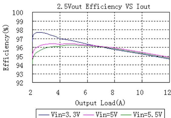
Figure 5: Converter efficiency vs. output current (2.5V out)
