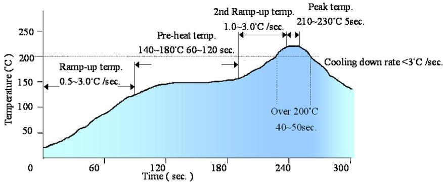
Note: The temperature refers to the pin of DCM, measured on the pin Vout joint.
