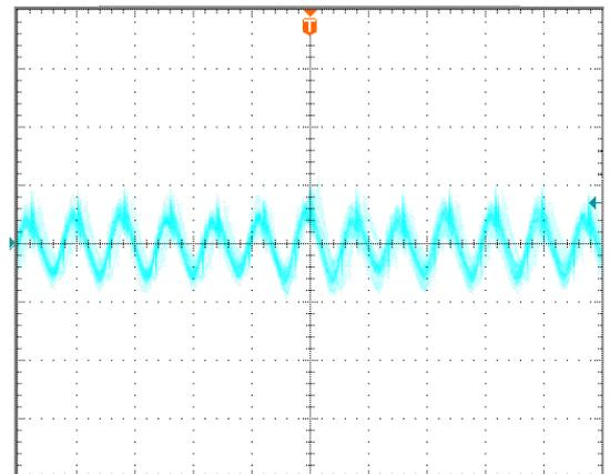
**Figure 10:** Output ripple & noise at 5Vin, 3.3V/12A out.
