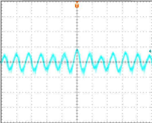
**Figure 9:** Output ripple & noise at 5Vin, 1.8V/12A out.
