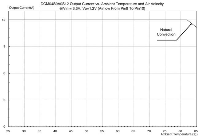
**Figure 41:** Output current vs. ambient temperature and air velocity @ Vin=3.3V, Vout=1.2V (Either Orientation)
