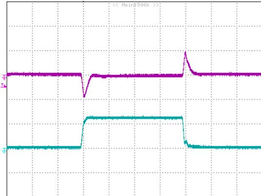
**Figure 19:** Typical transient response to step load change at  $2.5A/\mu S$  from 0% to 50% to 0% of  $I_o$ , max at  $5V_{in}$ ,  $0.6V_{out}$  (100uS/div) ( $C_{out} = 47\mu F$  ceramic). top trace:  $V_{out}$ , 0.2V/div; bottom trace:  $I_{out}$ :5A/div.
