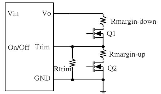
**Figure 33:** Circuit configuration for output voltage margining
