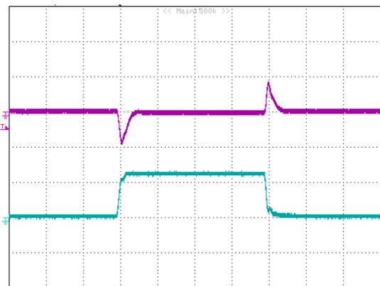
**Figure 21:** Typical transient response to step load change at  $2.5A/\mu S$  from 0% to 50% to 0% of  $I_o$ , max at  $5V_{in}$ ,  $1.8V_{out}$  (100uS/div) ( $C_{out} = 47\mu F$  ceramic). top trace:  $V_{out}$ , 0.2V/div; bottom trace:  $I_{out}$ :5A/div.
