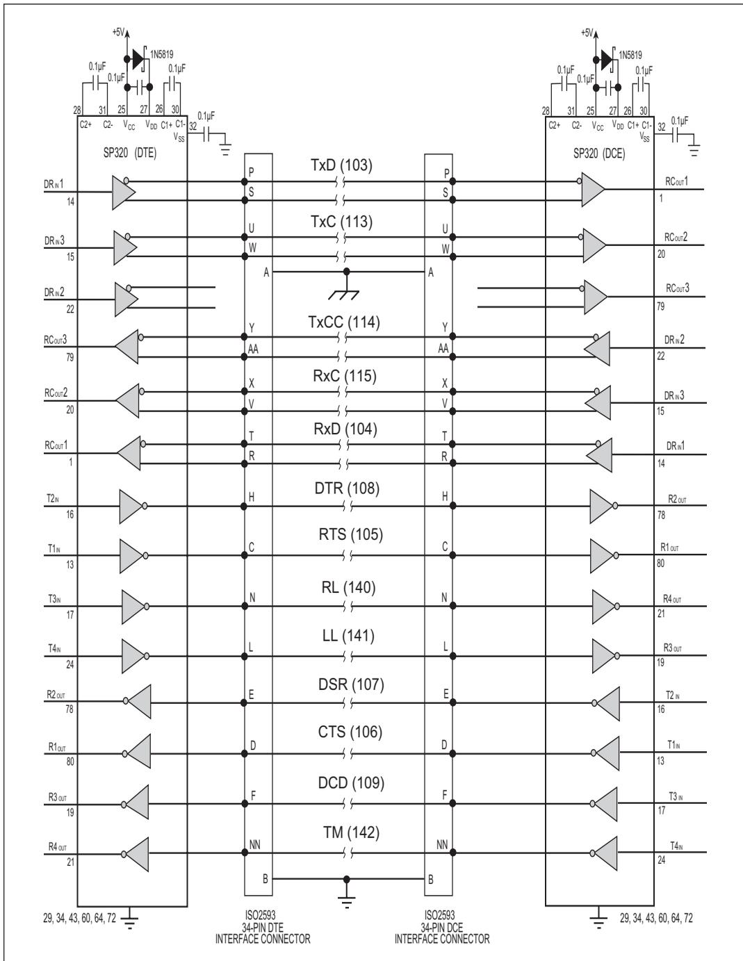
Figure 7. Typical DTE-DCE V.35 Connection with the SP320
