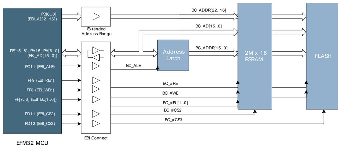
As shown in figure Figure 6.10, the PSRAM and FLASH devices are selected by the EBI\_CS2 and EBI\_CS3 signals, respectively. The PSRAM and Flash devices map to the EFM32's address space as following:
