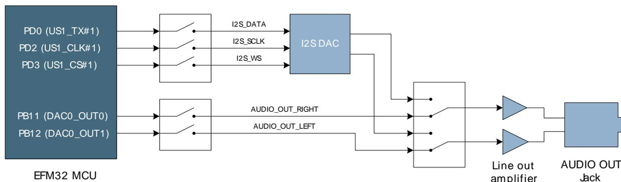
As shown in the block diagram above, a multiplexer is used to select between the two possible audio sources. The multiplexer and isolation switches are controlled by the board controller, and can be enabled by calling the appropriate function in the BSP API:
