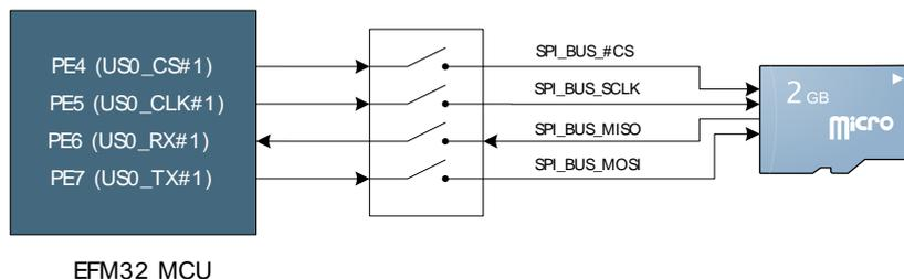
The microSD card slot can be connected to the EFM32 with the BSP function:
