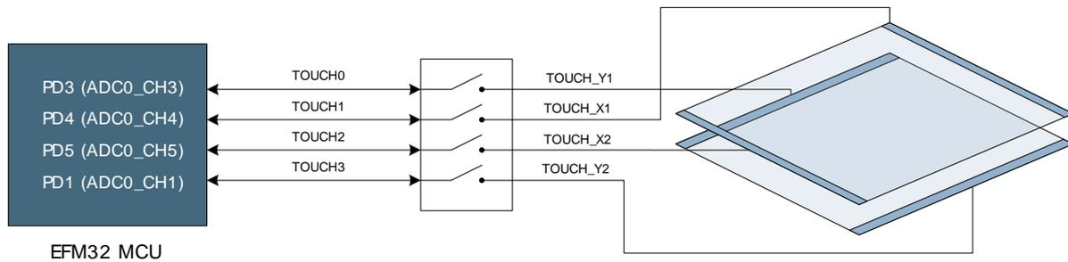
Figure shows how the resistive touch film is connected. When touched, the X-position can be read out by applying a voltage between the X1 and X2 electrodes and measuring the voltage on the Y1 or Y2 electrodes. Likewise, the Y-position can be read out by applying a voltage across the Y1 and Y2 electrodes and measuring the X1 or X2 electrodes.
