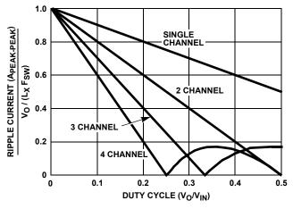
FIGURE 12. RIPPLE CURRENT vs DUTY CYCLE
