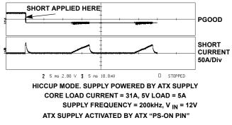
FIGURE 6. SHORT APPLIED TO SUPPLY AFTER POWER-UP
