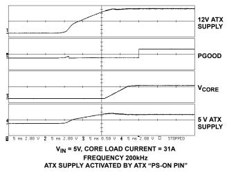
FIGURE 5. SUPPLY POWERED BY ATX SUPPLY
