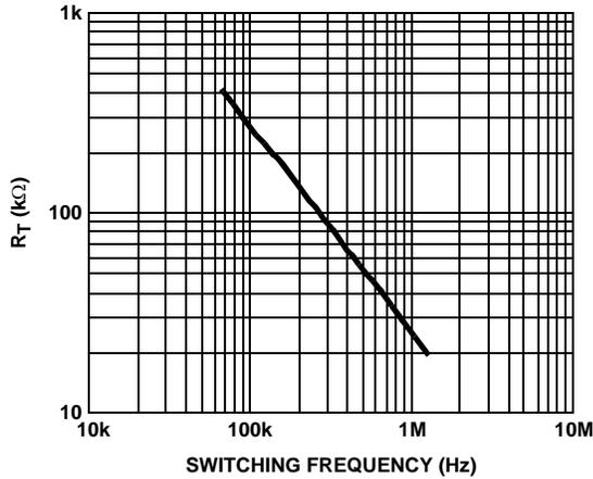
FIGURE 24.  $R_T$  vs SWITCHING FREQUENCY
