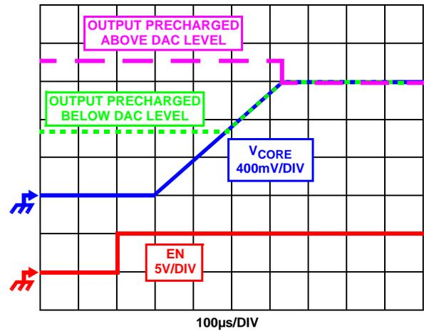
FIGURE 14. SOFT-START WAVEFORMS FOR ISL6323B-BASED MULTI-PHASE CONVERTER
