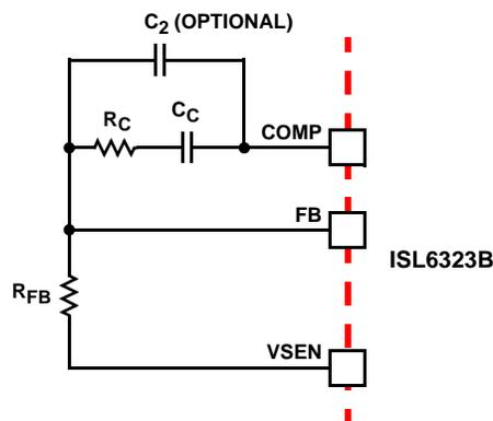
FIGURE 22. COMPENSATION CONFIGURATION FOR LOAD-LINE REGULATED ISL6323B CIRCUIT
