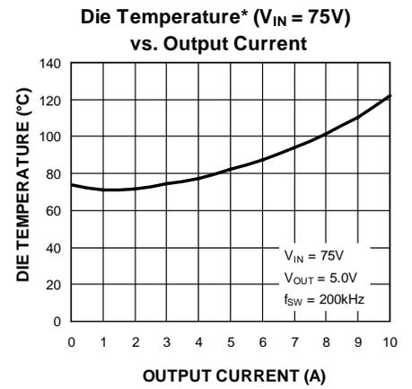
\* **Case Temperature:** The temperature measurement was taken at the hottest point on the MIC2103 case mounted on a 5 square inch PCB, see Thermal Measurement section. Actual results will depend upon the size of the PCB, ambient temperature and proximity to other heat emitting components.
