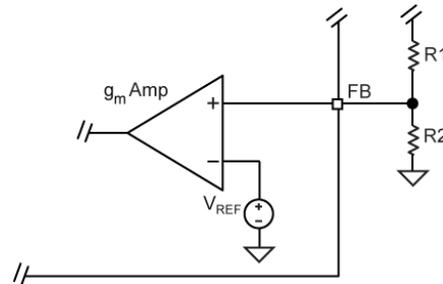
Figure 7. Voltage-Divider Configuration
