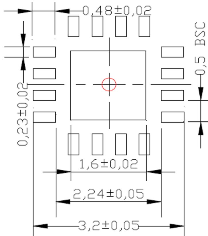
**Red circle** indicates Thermal Via. Size should be .300mm – .350mm in diameter and it should be connected to GND plane for maximum thermal performance.
