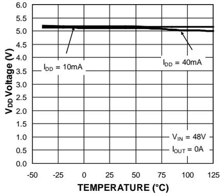
**V<sub>DD</sub> UVLO Threshold vs. Temperature**
