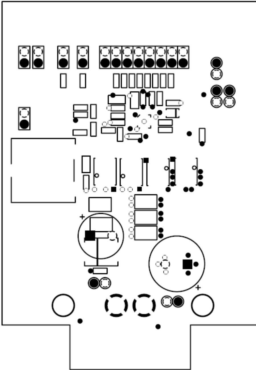
Figure 11. MIC2103/04 Evaluation Board Mid-Layer 1 (Ground Plane)
