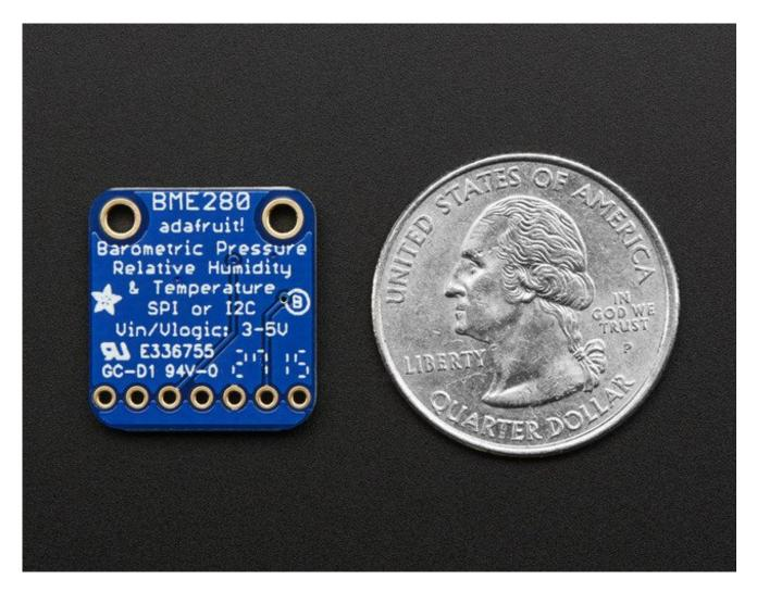
The BME280 is the next-generation of sensors from Bosch, and is the upgrade to the BMP085/BMP180/BMP183 - with a low altitude noise of 0.25m and the same fast conversion time. It has the same specifications, but can use either I2C *or* SPI. For simple easy wiring, go with I2C. If you want to connect a bunch of sensors without worrying about I2C address collisions, go with SPI.
