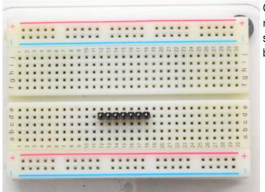
Cut the strip to length if necessary. It will be easier to solder if you insert it into a breadboard - **long pins down**
