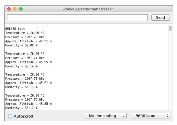
**Temperature** is calculated in degrees C, you can convert this to F by using the classic F = C \* 9/5 + 32 equation.
