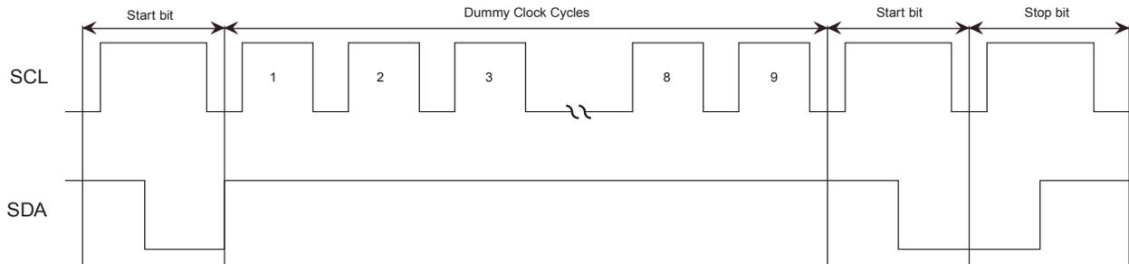
The ATAES132A requires that the clock be pulled low between the Start condition and the Stop condition at the end of the sequence, as illustrated in Figure J-7. It will not reset if this clock transition is omitted. See Appendix J.4, I<sup>2</sup>C Interface Synchronization Procedure for detailed I<sup>2</sup>C interface resynchronization instructions.
