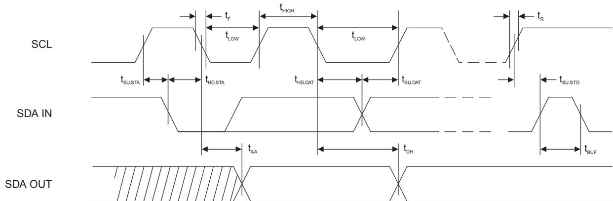
Figure J-10. I<sup>2</sup>C Write Cycle Timing
