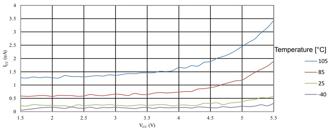
**Figure 35-14 ATmega328PB: Power-Down Supply Current vs. V<sub>CC</sub> (Watchdog Timer Enabled)**
