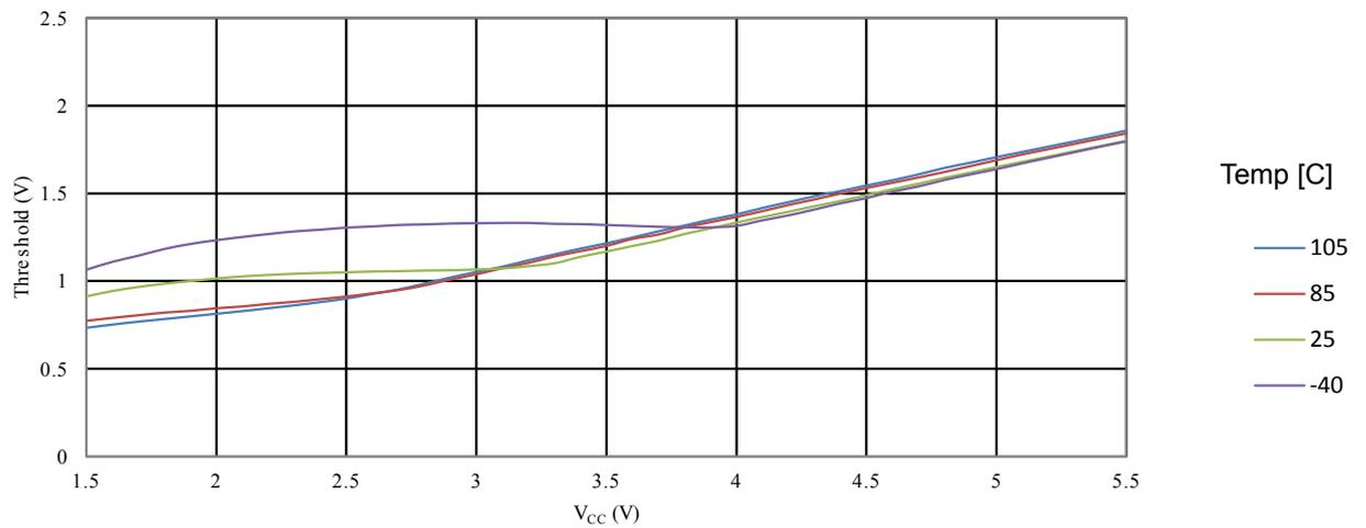
**Figure 35-30 ATmega328PB Reset Input Threshold Voltage vs.  $V_{CC}$  ( $V_{IL}$ , I/O Pin read as '0')**
