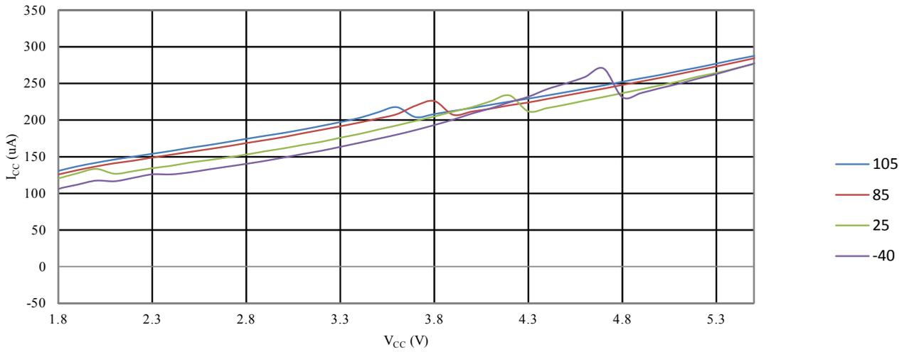
Figure 35-48 ATmega328PB: Analog Comparator Current vs. V<sub>CC</sub>
