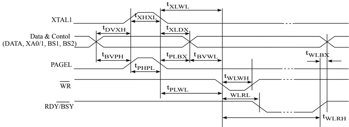
**Figure 34-7 Parallel Programming Timing, Loading Sequence with Timing Requirements**
