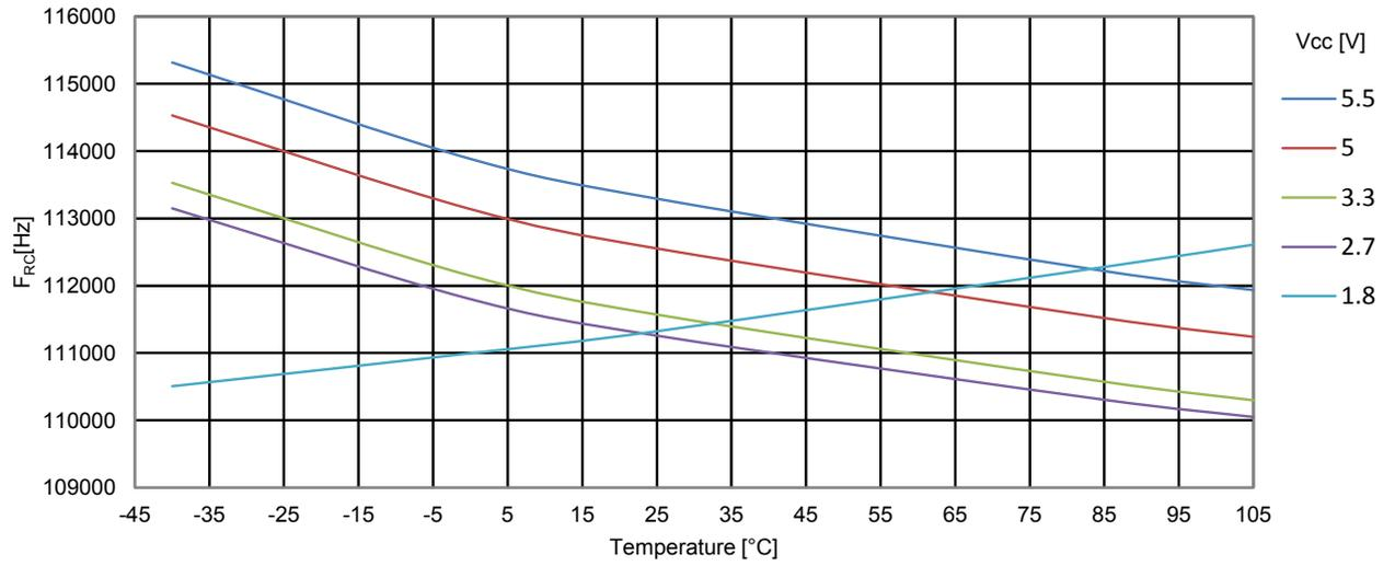
Figure 35-42 ATmega328PB: Watchdog Oscillator Frequency vs.  $V_{CC}$
