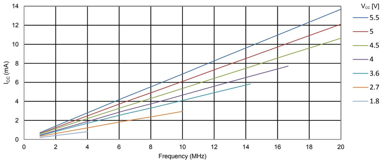
Figure 35-3 ATmega328PB: Active Supply Current vs.  $V_{CC}$  (Internal RC Oscillator, 128kHz)
