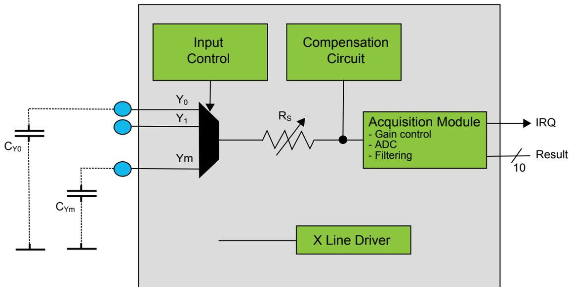
**Note:** For 328PB the  $R_s = 20\text{-}100\text{ K}\Omega$ .
