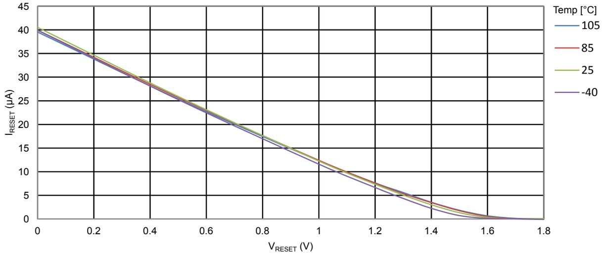
**Figure 35-20 ATmega328PB: Reset Pull-up Resistor Current vs. Reset Pin Voltage**
