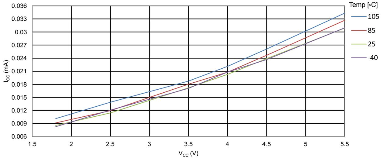
**Figure 35-11 ATmega328PB: Idle Supply Current vs.  $V_{CC}$  (Internal RC Oscillator, 1MHz)**
