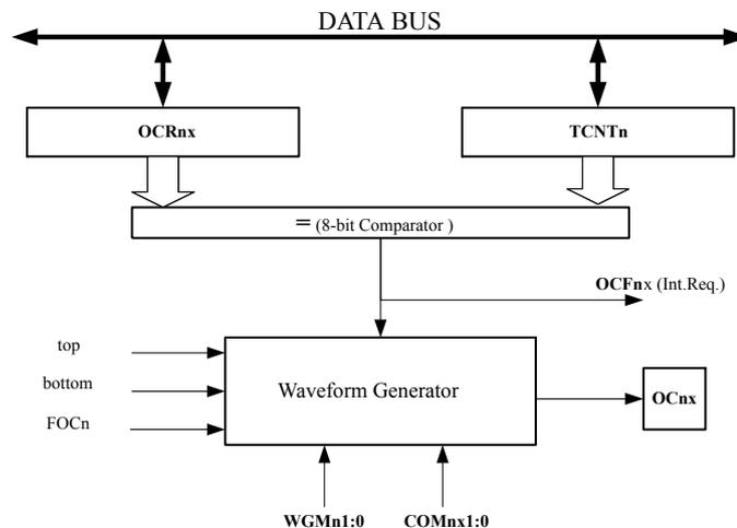
The OCR<sub>n</sub> Registers are double buffered when using any of the Pulse Width Modulation (PWM) modes. When double buffering is enabled, the CPU has access to the OCR<sub>0</sub>x Buffer Register. The double buffering synchronizes the update of the OCR<sub>n</sub> Compare Registers to either top or bottom of the counting sequence. The synchronization prevents the occurrence of odd-length, non-symmetrical PWM pulses, thereby making the output glitch-free.
