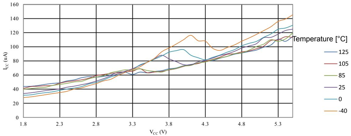
Figure 35-49 ATmega328PB: AREF External Reference Current vs. V<sub>CC</sub>
