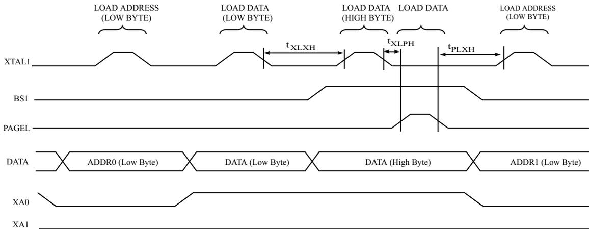
**Note:** The timing requirements shown in [Parallel Programming Characteristics](#) on page 386 (i.e.,  $t_{DVXH}$ ,  $t_{XHXL}$ , and  $t_{XLDX}$ ) also apply to loading operation
