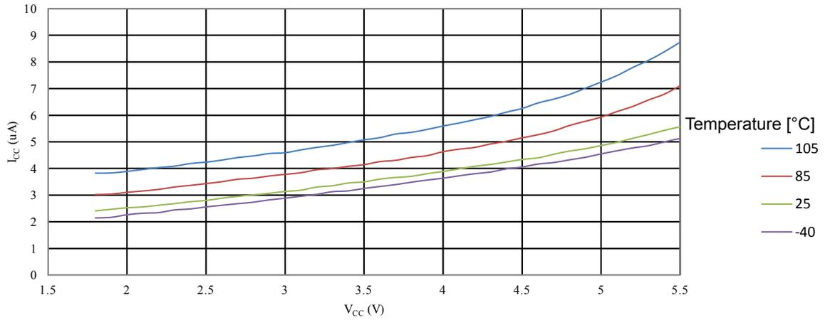
**Figure 35-15 ATmega328PB: Power-Down Supply Current vs. V<sub>CC</sub> (AREF, VCCDIV2)**
