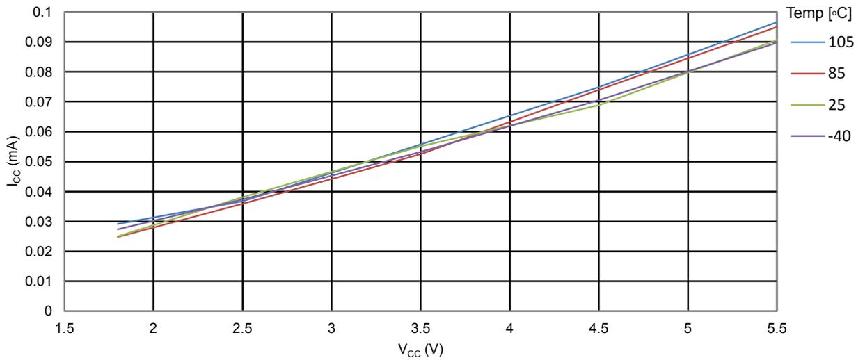
Figure 35-4 ATmega328PB: Active Supply Current vs.  $V_{CC}$  (Internal RC Oscillator, 1MHz)
