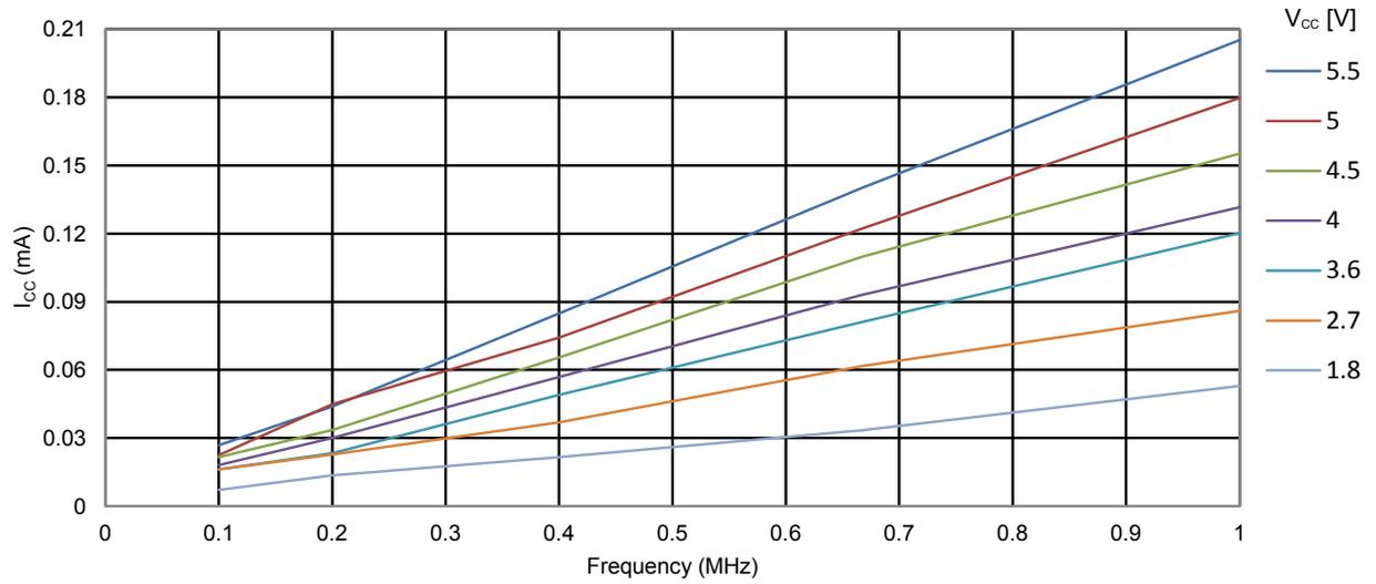
Figure 35-9 ATmega328PB: Idle Supply Current vs. Frequency (1-20MHz)
