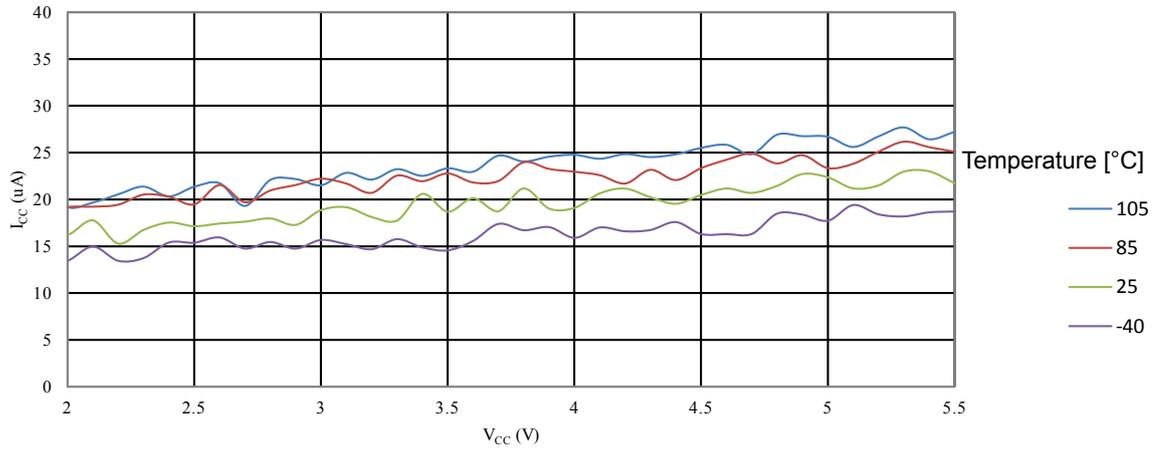
Figure 35-51 ATmega328PB: Programming Current vs. Vcc
