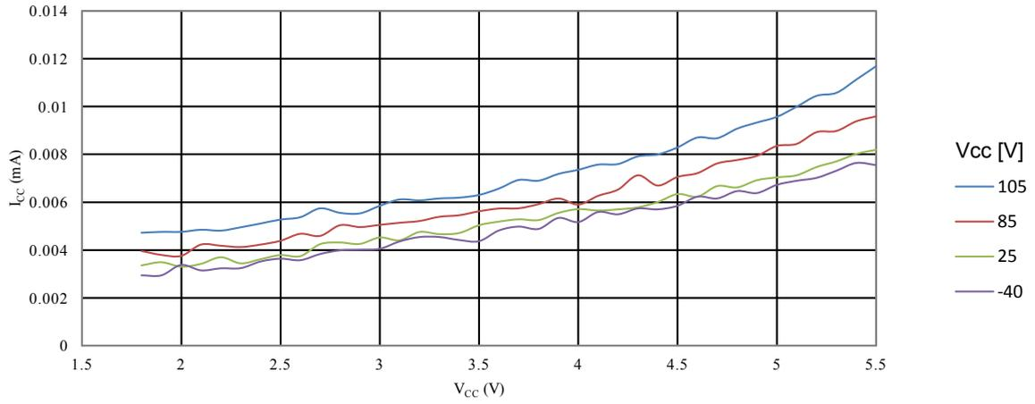
Figure 35-55 ATmega328PB: Minimum Reset Pulse Width vs. V<sub>CC</sub>
