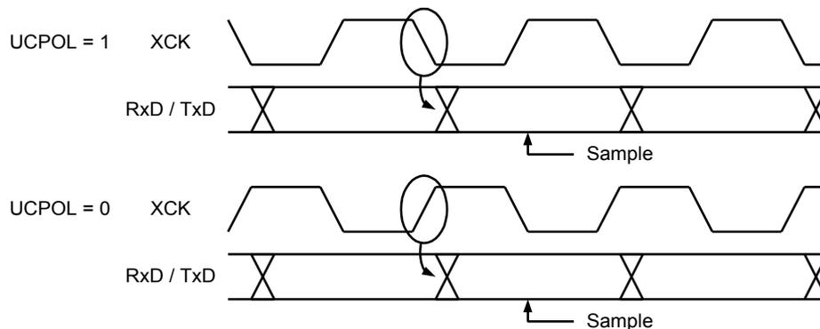
The UCPOL bit UCRSC selects which XCKn clock edge is used for data sampling and which is used for data change. As the above timing diagram shows, when UCPOL is zero, the data will be changed at
