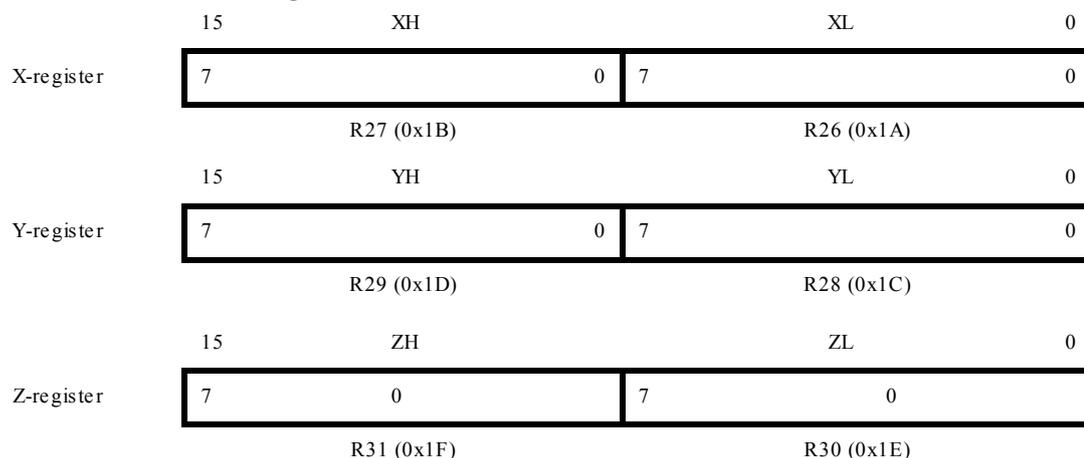
In the different addressing modes these address registers have functions as fixed displacement, automatic increment, and automatic decrement. See *Instruction Set Summary* for details.
