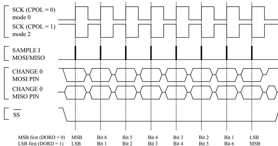
**Figure 24-4 SPI Transfer Format with CPHA = 1**
