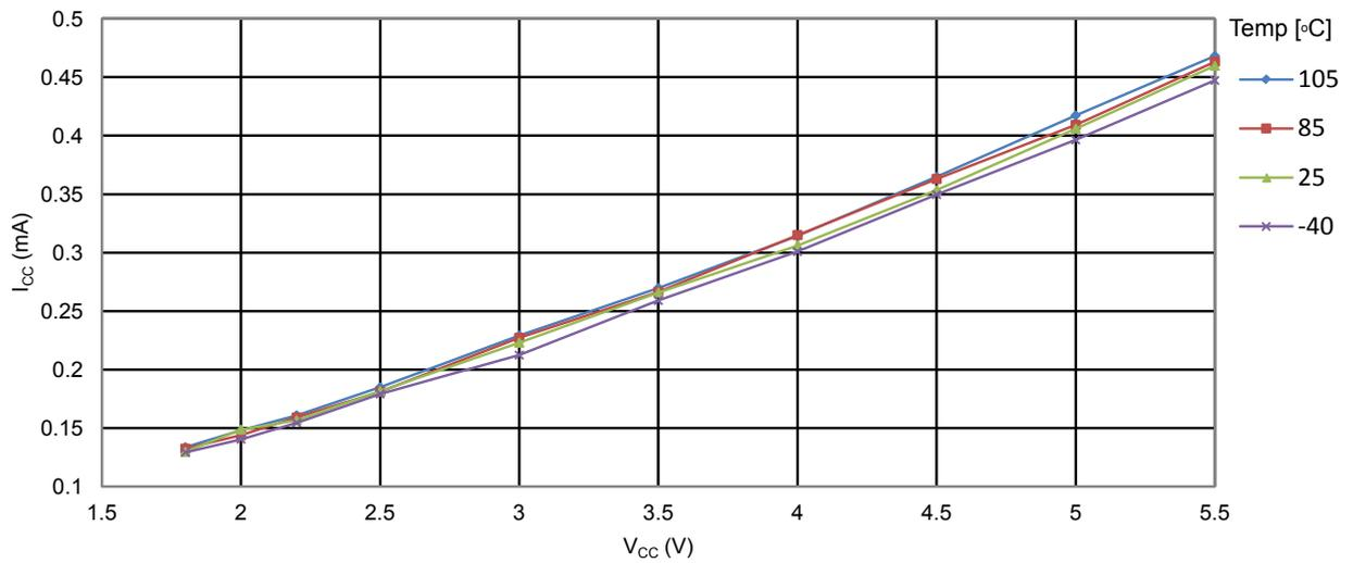
**Figure 35-12 ATmega328PB: Idle Supply Current vs.  $V_{CC}$  (Internal RC Oscillator, 8MHz)**
