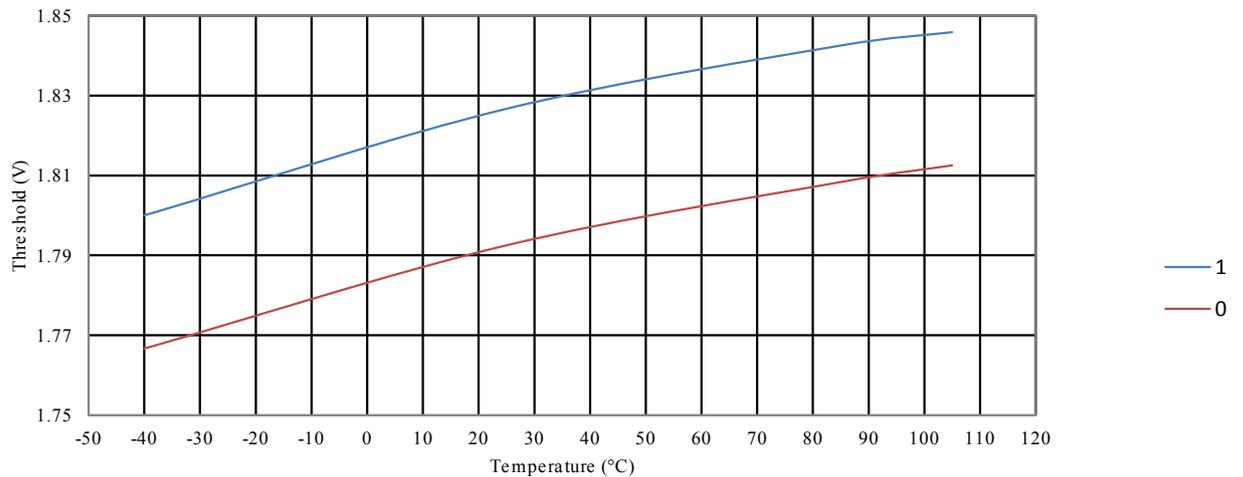
**Figure 35-33 ATmega328PB: BOD Thresholds vs. Temperature (BODLEVEL is 2.7V)**
