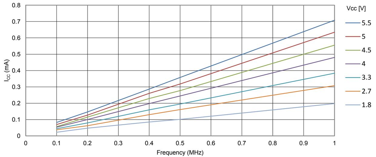
Figure 35-2 ATmega328PB: Active Supply Current vs. Frequency (1-20MHz)
