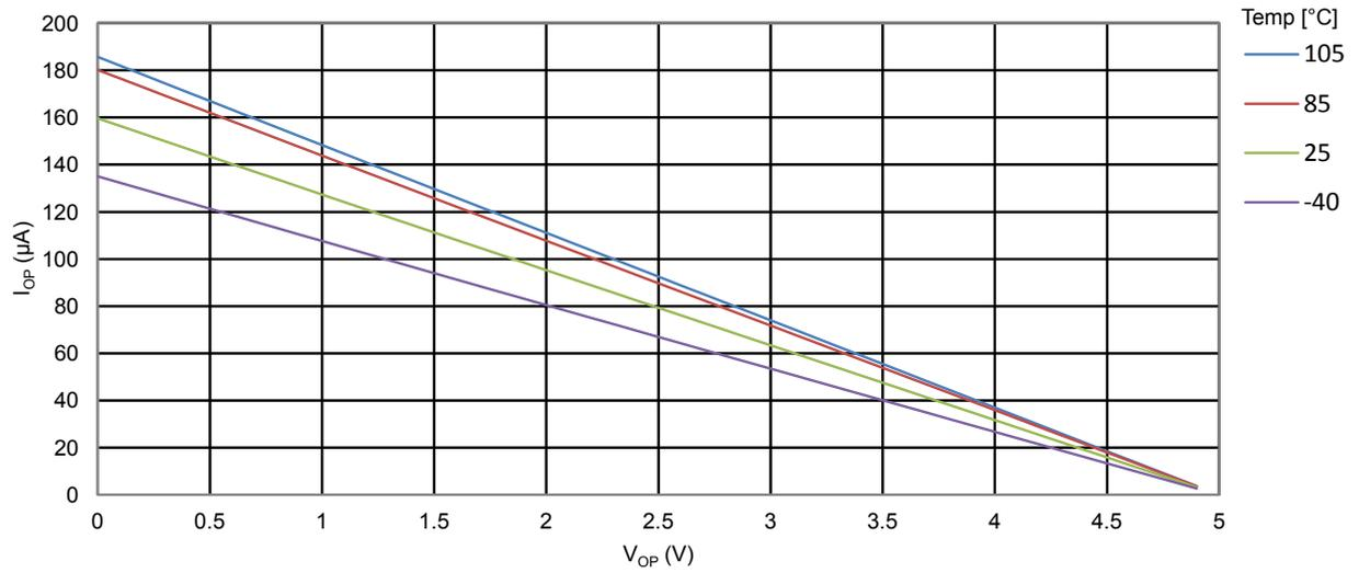
**Figure 35-19 ATmega328PB: Reset Pull-up Resistor Current vs. Reset Pin Voltage**
