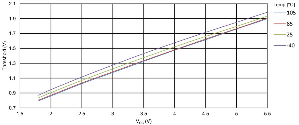
**Figure 35-28 ATmega328PB I/O Pin Input Hysteresis vs.  $V_{CC}$**
