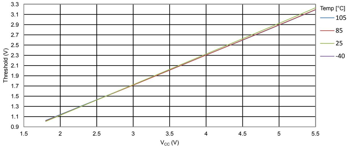
**Figure 35-27 ATmega328PB I/O Pin Input Threshold Voltage vs.  $V_{CC}$  ( $V_{IL}$ , I/O Pin read as '0')**
