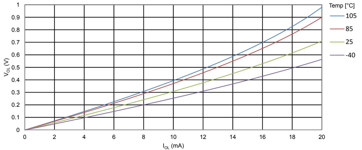
Figure 35-23 ATmega328PB: I/O Pin Output Voltage vs. Sink Current ( $V_{CC} = 5V$ )
