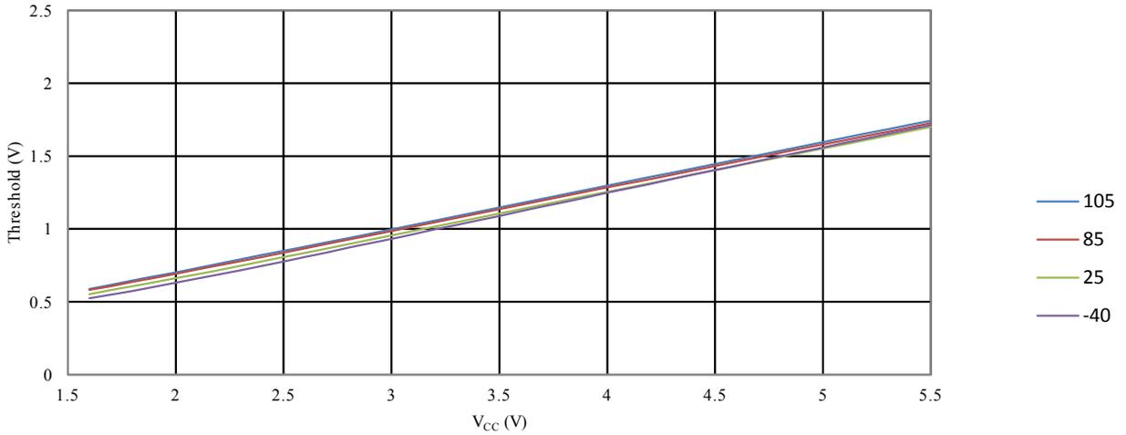
**Figure 35-31 ATmega328PB Reset Pin Input Hysteresis vs.  $V_{CC}$**
