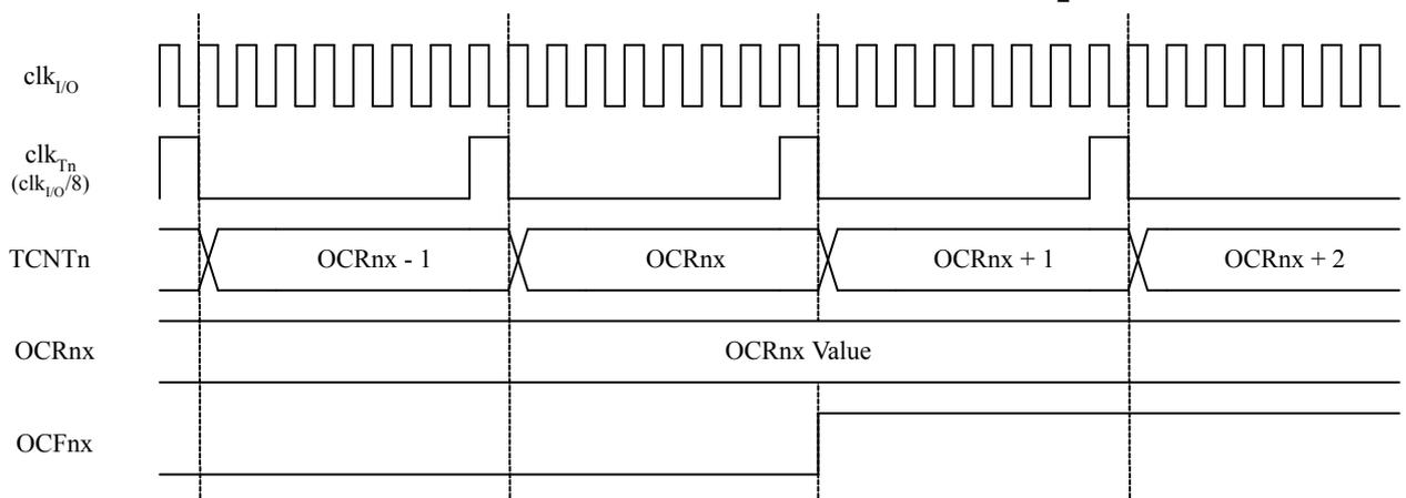
The following figure shows the setting of OCF2A and the clearing of TCNT2 in CTC mode.
