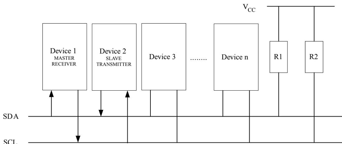
A START condition is sent by writing to the TWI Control register (TWCRn) a value of the type TWCRn=1x10x10x:
