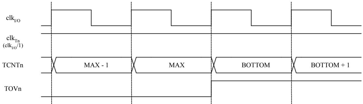
The following figure shows the same timing data, but with the prescaler enabled.
