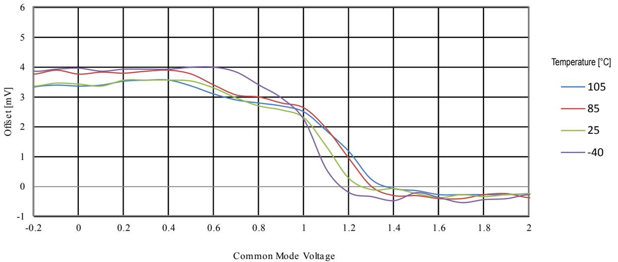
**Figure 35-39 ATmega328PB AC Offset vs. Common Volaltage ( $V_{CC} = 3.0V$ )**
