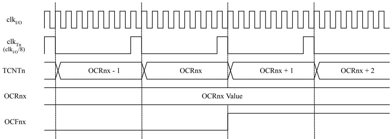
The next figure shows the setting of OCF0A and the clearing of TCNT0 in CTC mode and fast PWM mode where OCR0A is TOP.
