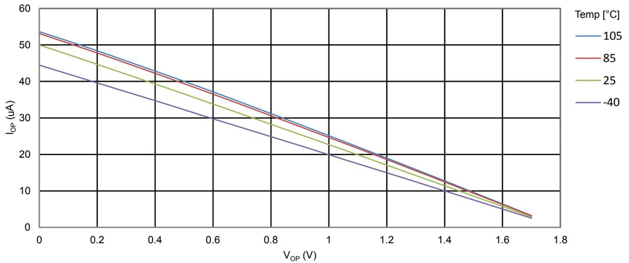
Figure 35-17 ATmega328PB: I/O Pin Pull-up Resistor Current vs. Input Voltage ( $V_{CC} = 2.7V$ )
