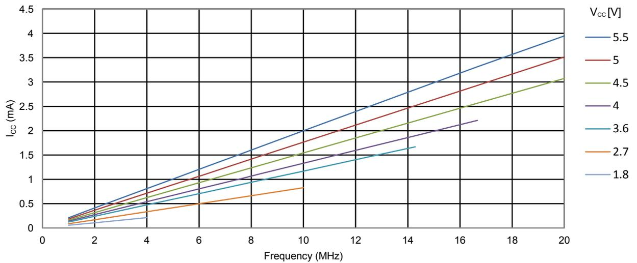
Figure 35-54 ATmega328PB: Reset Supply Current vs. V<sub>CC</sub> (Excluding current through Reset Pullup)
