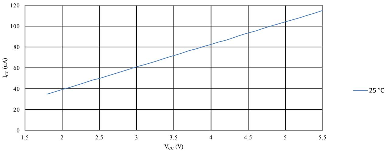
Figure 35-50 ATmega328PB: Brownout Detector Current vs. Vcc
