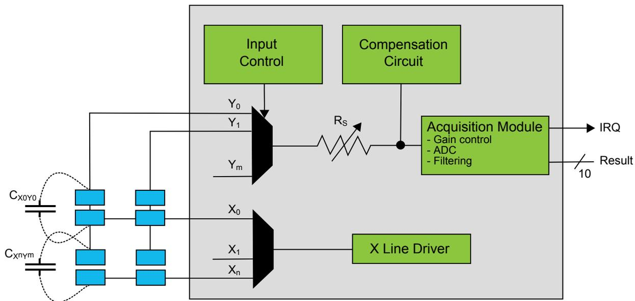
**Note:** For 328PB the  $R_s = 20\text{-}100\text{ K}\Omega$ .
