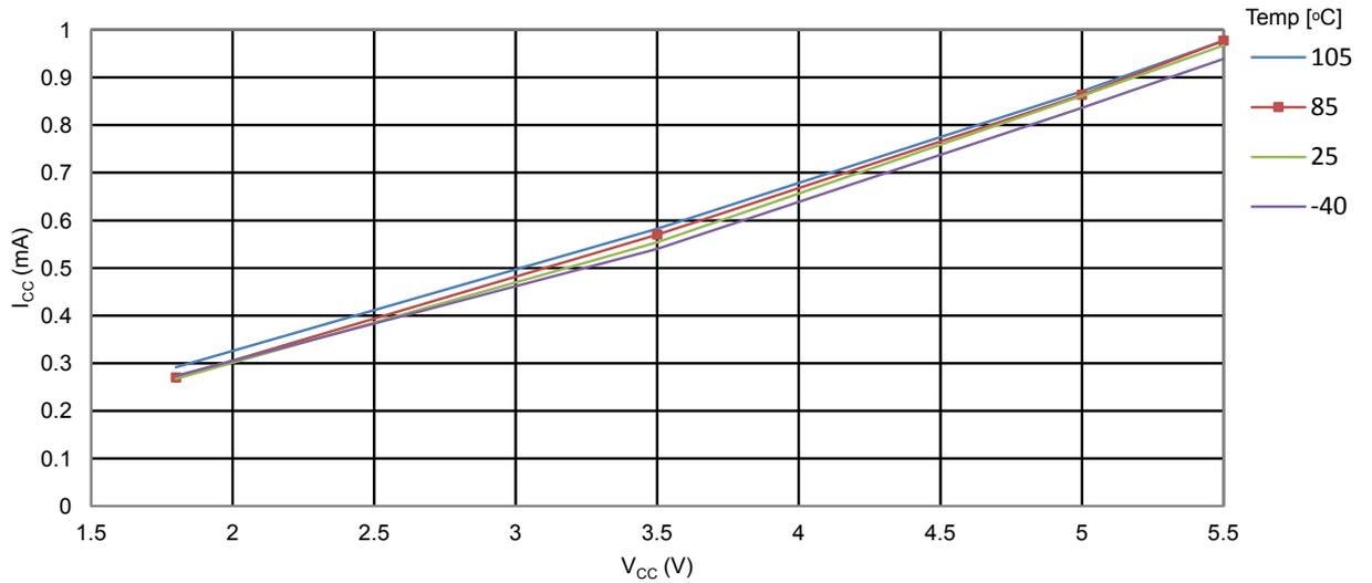
**Figure 35-5 ATmega328PB: Active Supply Current vs.  $V_{CC}$  (Internal RC Oscillator, 8MHz)**
