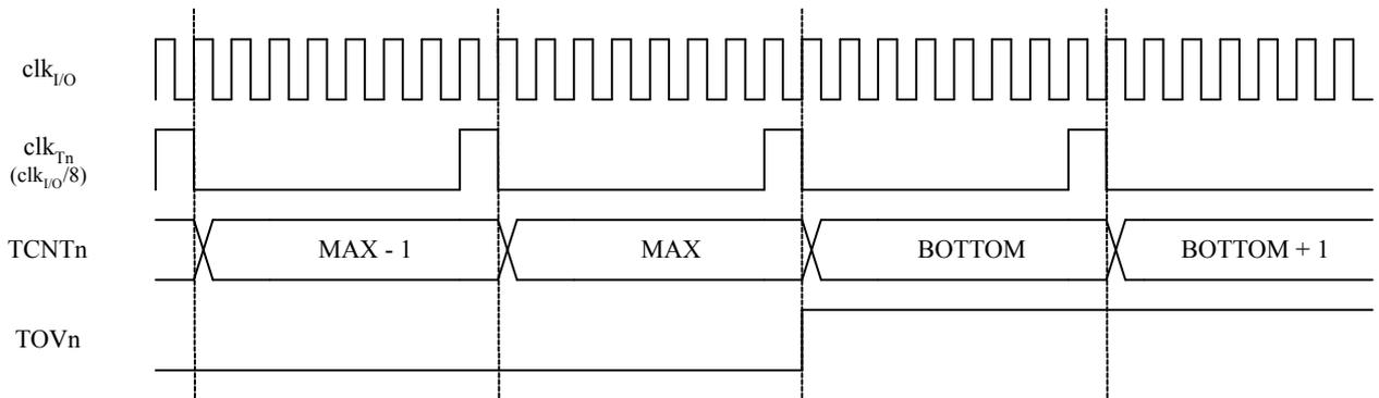
The next figure shows the setting of OCF0B in all modes and OCF0A in all modes (except CTC mode and PWM mode where OCR0A is TOP).
