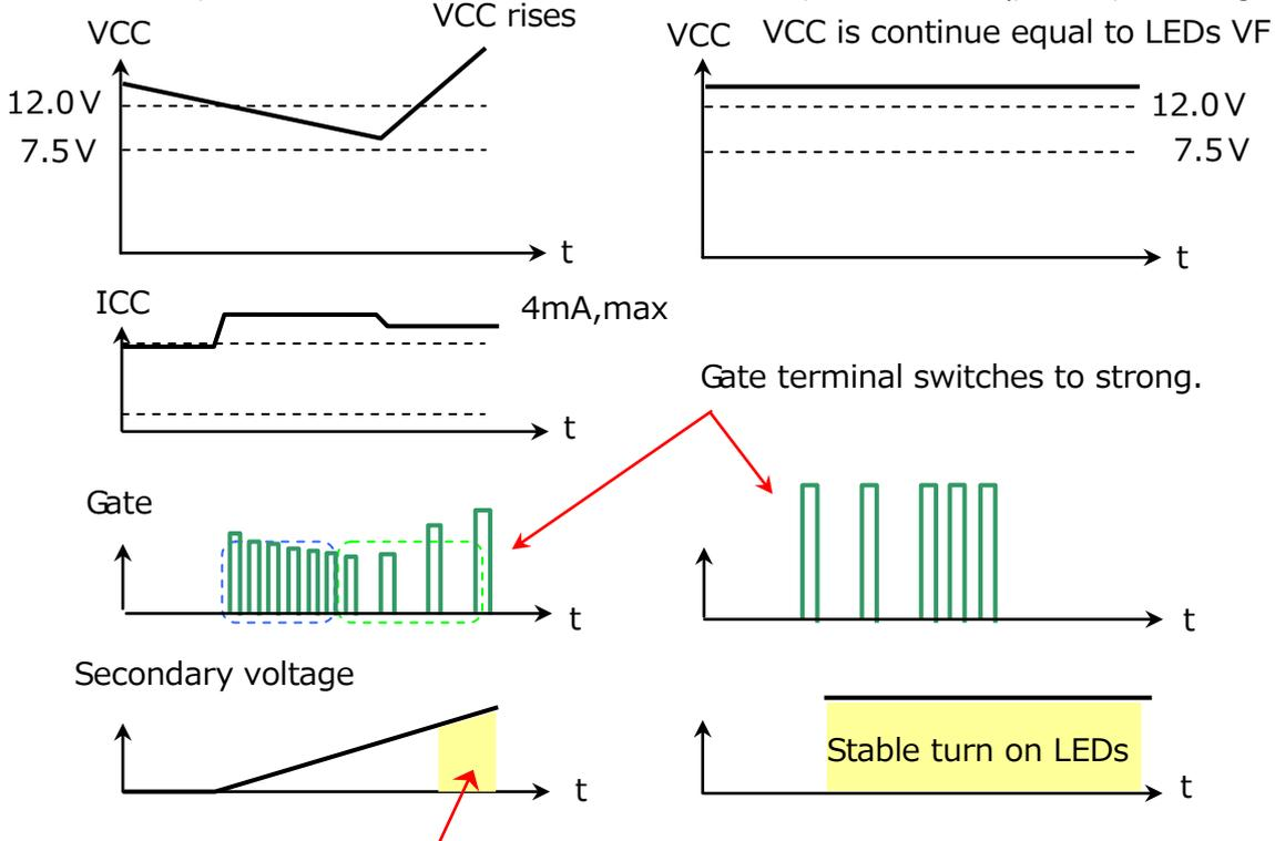
When the secondary voltage over LED's VF, LED start to turn it on.
