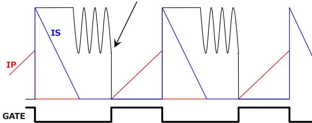
This resonance-amplitude is related to the VF of the LED and primary secondary turn-ratio Ntr.
