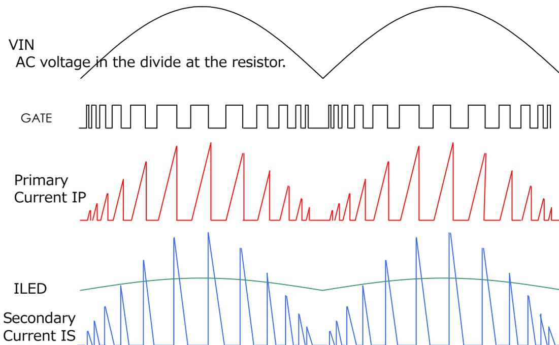
Because the main system is single stage PFC, the LED current waveform of the secondary side includes a ripple. To make LED current waveform smoother, it makes a secondary output capacitor big. The GATE pin is modulating a frequency.
