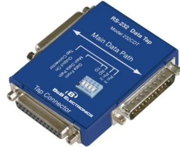
The small switch is used to program the Tap Connector. The bottom two switches pick Receive Data (RD) or Transmit Data (TD) to be sent to the Tap Connector. (See the markings near the switch.) When the RD switch is on, only mainline Receive Data is sent to the Tap Connector. When the TD switch is on, only mainline Transmit Data is sent to the Tap Connector. When both switches are on, both the Transmit Data and the Receive Data are sent to the Tap Connector.
