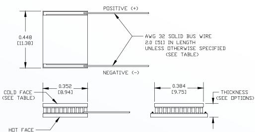
Ceramic Material 96% Alumina Ceramics Solder Construction: 138°C, Bismuth Tin
