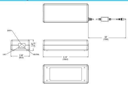
1.47" (H) x 2.56" (W) x 6.14" (L) 37.2 mm (H) x 65.0 mm (W) x 156.0 mm (L) AC Input Connector: IEC320, C6 AC Input power cord sold separately
