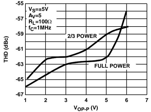
FIGURE 30. DIFFERENTIAL TOTAL HARMONIC DISTORTION vs OUTPUT AMPLITUDE
