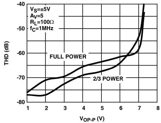
FIGURE 24. DIFFERENTIAL TOTAL HARMONIC DISTORTION vs OUTPUT AMPLITUDE
