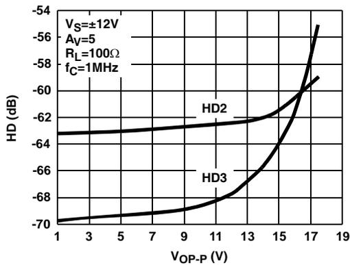
FIGURE 27. DIFFERENTIAL HARMONIC DISTORTION vs OUTPUT AMPLITUDE (2/3 POWER)
