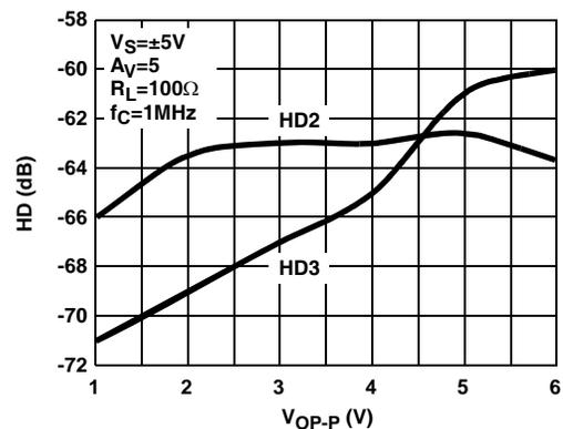
FIGURE 28. DIFFERENTIAL HARMONIC DISTORTION vs OUTPUT AMPLITUDE (2/3 POWER)
