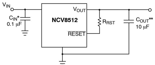
\* $C_{\text{IN}}$  required if regulator is located far from the power supply filter.
