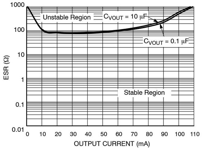
Figure 9. Output Stability with Output Capacitor Change
