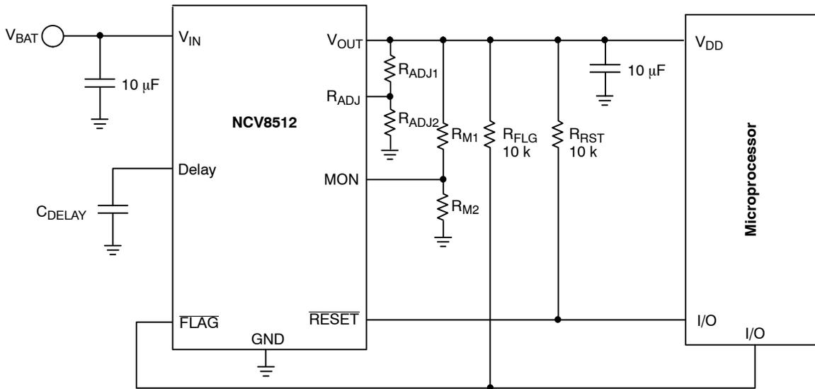
**Figure 1. Application Diagram**
