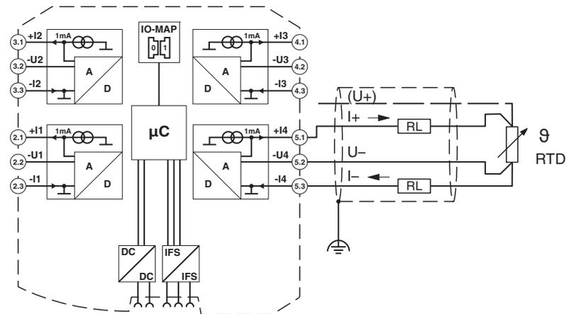
Figure 10 4-wire connection technology
