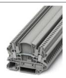
Feed-through terminal block, Connection method: Screw connection, Cross section: 0.14 mm² - 6 mm², AWG: 26 - 10, Width: 6.2 mm, Color: gray, Mounting type: NS 35/7,5, NS 35/15
