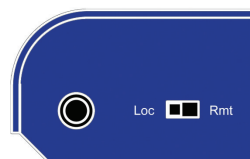
The DIP switch is on top of the device.
