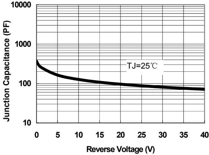
Fig.1-Typical Junction Capacitance
