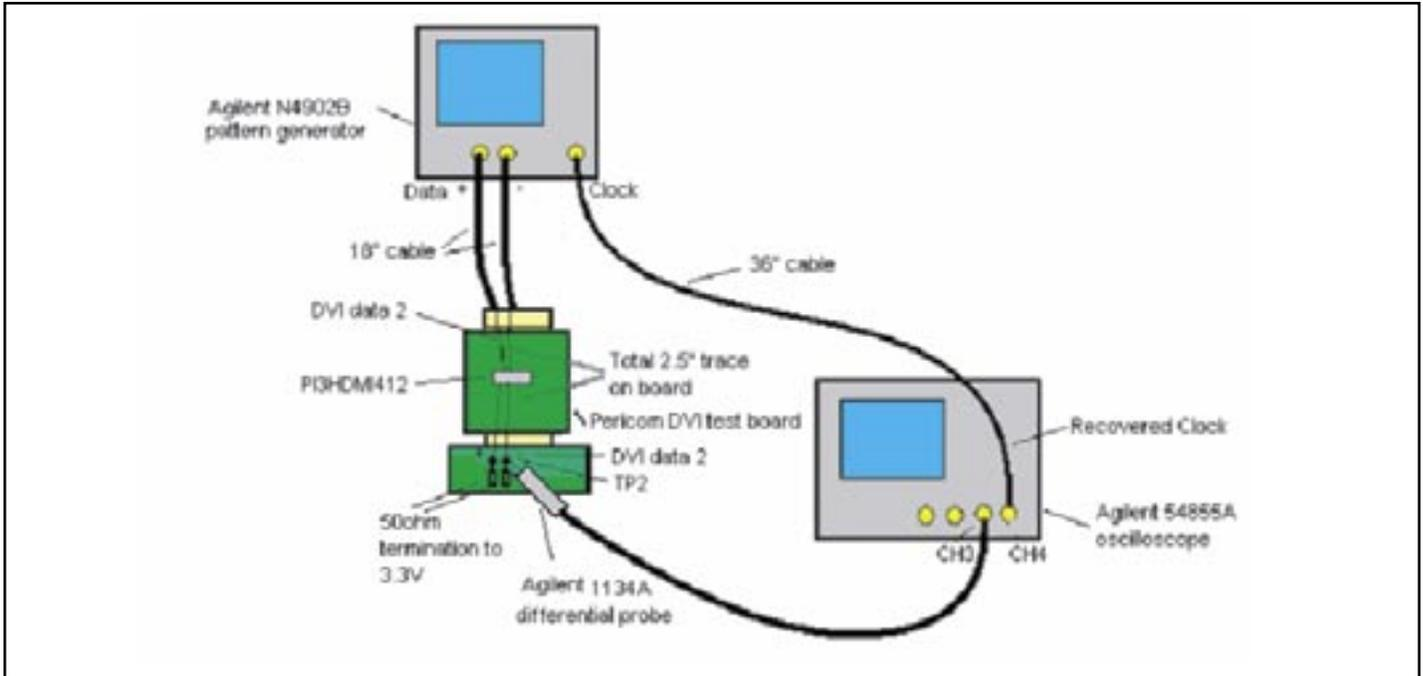
Figure 1. TMDS TP2 Tx eye compliance test setup
