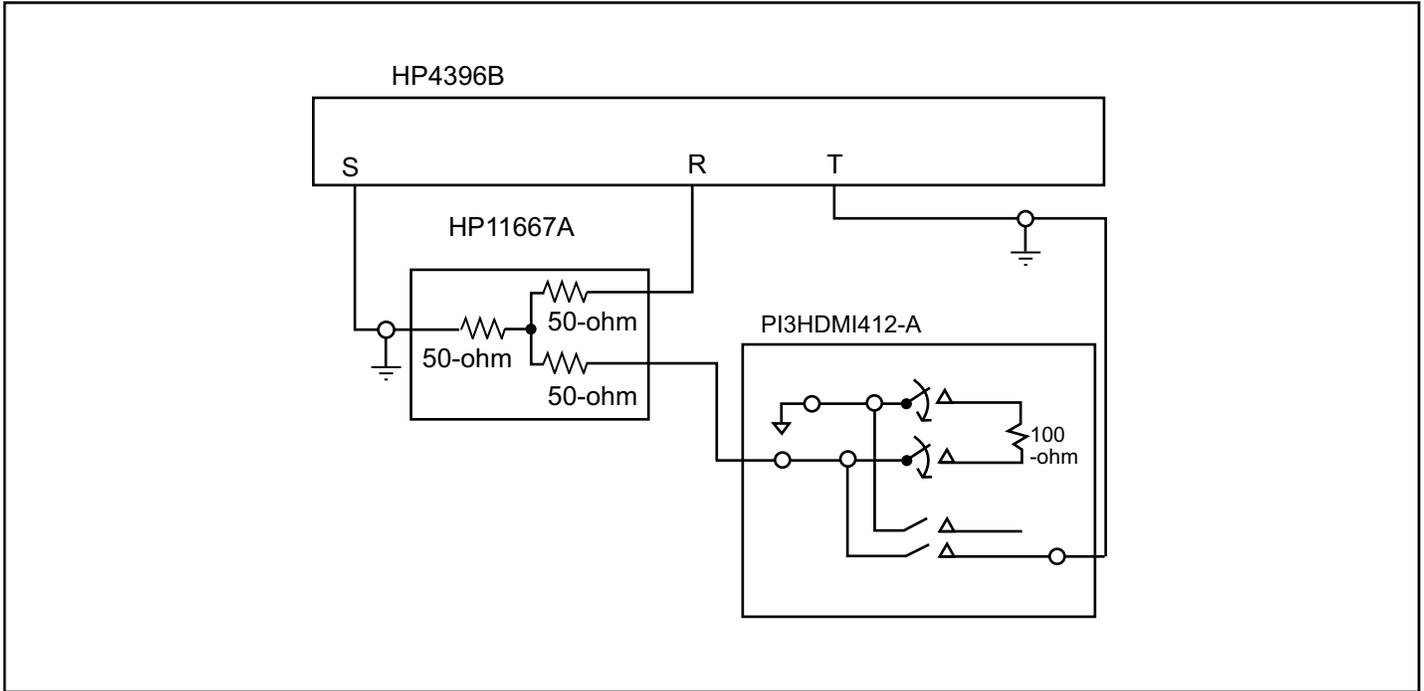
Fig 2. Off-isolation setup
