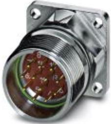
Device connector, front mounting, straight, Screw locking, M23, Number of positions: 12, Type of contact: Male connector, Crimp connection, Axial O-ring, 4xØ3,2, Shielded: Yes
