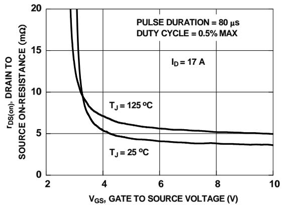
Figure 16. On-Resistance vs Gate to Source Voltage
