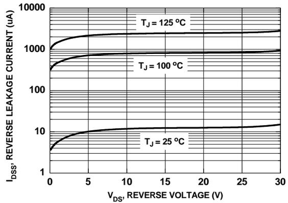
Figure 26. SyncFET<sup>™</sup> Body Diode Reverse Leakage vs. Drain-Source Voltage
