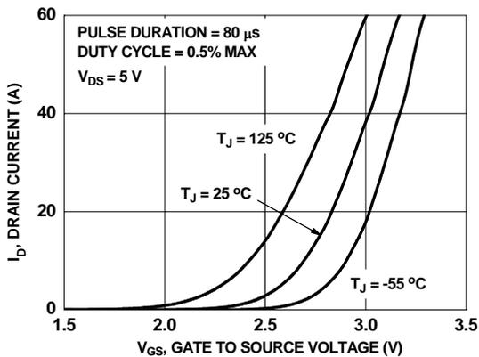
Figure 17. Transfer Characteristics
