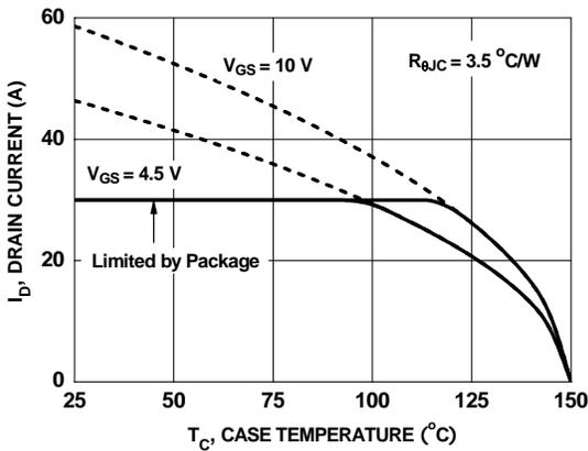
**Figure 9. Maximum Continuous Drain Current vs Case Temperature**
