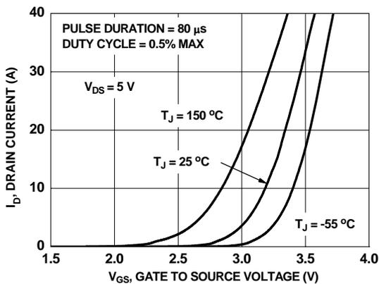
Figure 5. Transfer Characteristics
