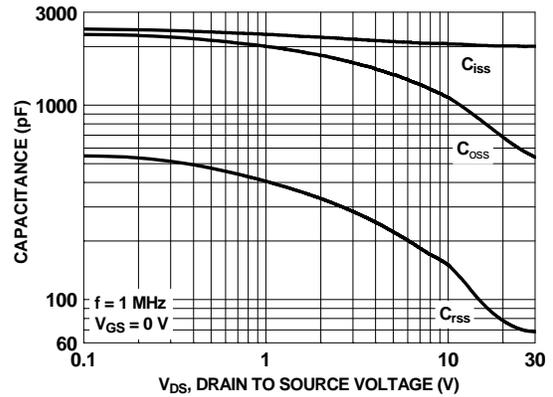
Figure 20. Capacitance vs Drain to Source Voltage
