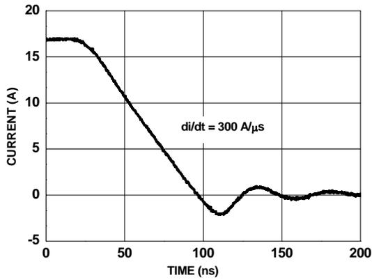
Figure 25. FDMS7602S SyncFET<sup>™</sup> Body Diode Reverse Recovery Characteristic
