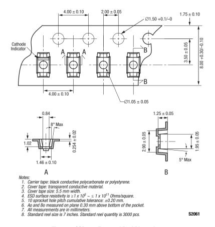
Figure 4. SOD-323 Tape and Reel Dimensions
