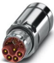
Coupling connector, straight long, shielded: yes, Screw locking, M23, Number of positions: 8+4+PE / 3+N +PE, Type of contact: Pin, Crimp connection, Cable diameter: 15 mm ... 18 mm
