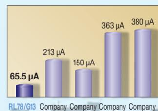
Operating current comparison during clock operation (32.768 kHz, RTC + LVD)
