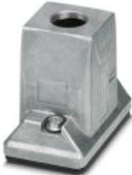
HEAVYCON ADVANCE sleeve housing, B6, with stainless steel screw locking (Allen screw), salt-water-resistant aluminum, height 74 mm, with 1x M25 thread, straight cable outlet, without surface; conductive seal (EMC properties)
