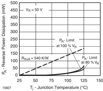
Fig. 1 - Max. Reverse Power Dissipation vs. Junction Temperature
