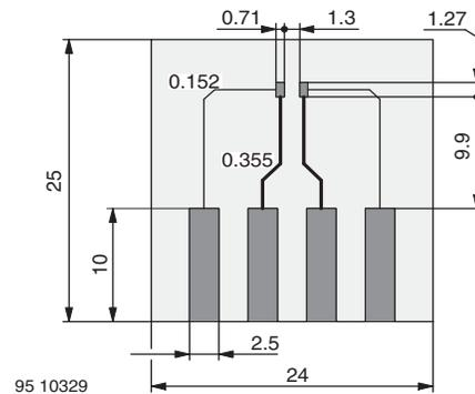
Fig. 5 - Board for  $R_{thJA}$  Definition (in mm)
