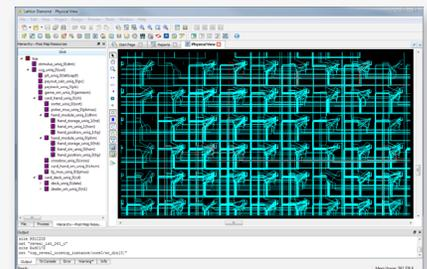
A detailed, read-only view of the physical routing of paths for a more detailed understanding of timing issues.
