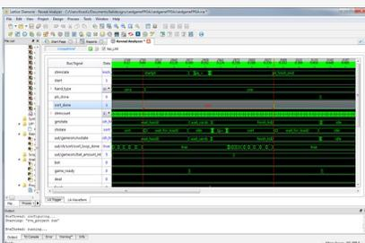
The Reveal Hardware Debugger uses a signal-centric model that allows easy insertion of embedded logic analyzer debug hardware for real-time analysis.
