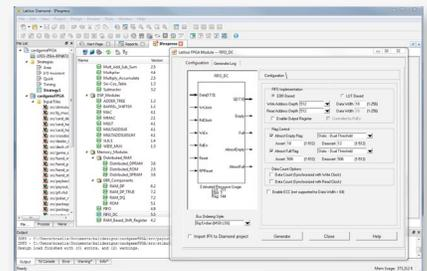
An interface to the Lattice catalog of modules and IP optimized for Lattice devices.
