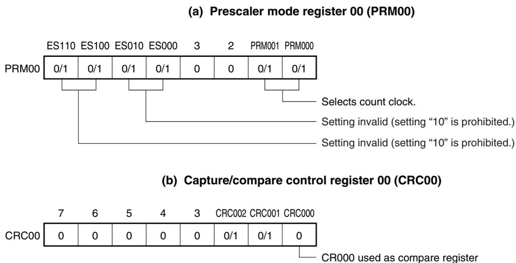
Figure 6-27. Control Register Settings in Square-Wave Output Mode (2/2)
