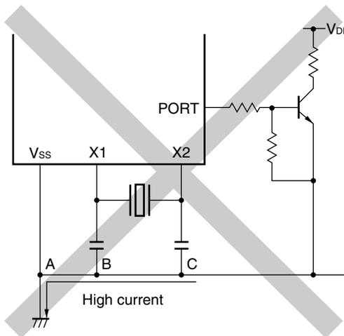
Figure 5-7. Examples of Incorrect Resonator Connection (2/2)
