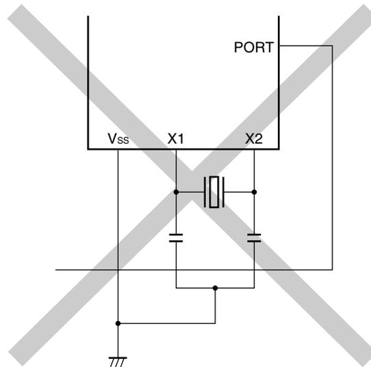
(c) Wiring near high fluctuating current
