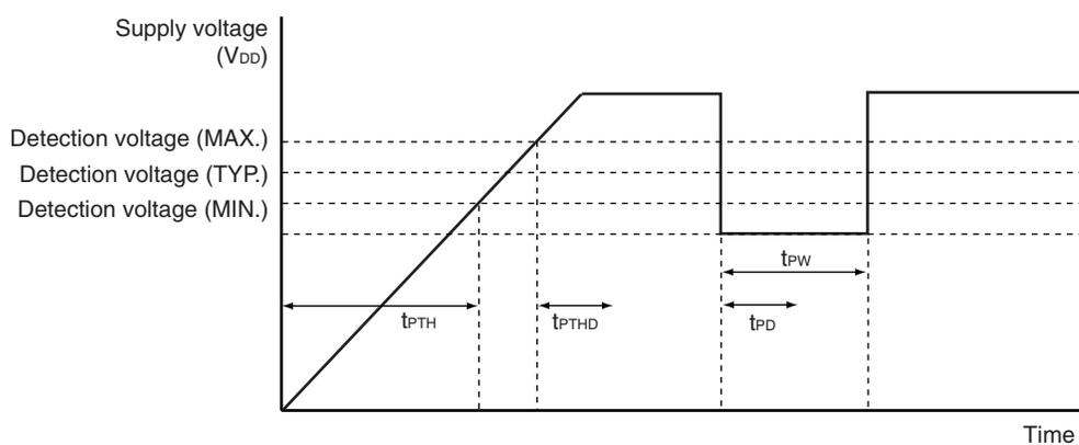
LVI Circuit Characteristics ( $T_A = -40$  to  $+125^\circ\text{C}$ )
