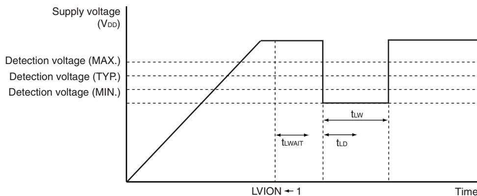
Data Memory STOP Mode Low Supply Voltage Data Retention Characteristics ( $T_A = -40$  to  $+125^\circ\text{C}$ )
