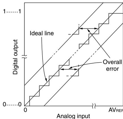
Figure 10-14. Quantization Error
