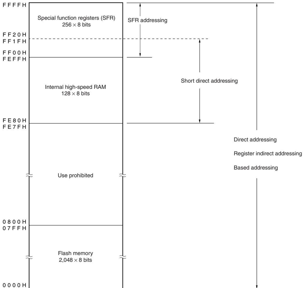
Figure 3-5. Data Memory Addressing ( $\mu$ PD78F9222)
