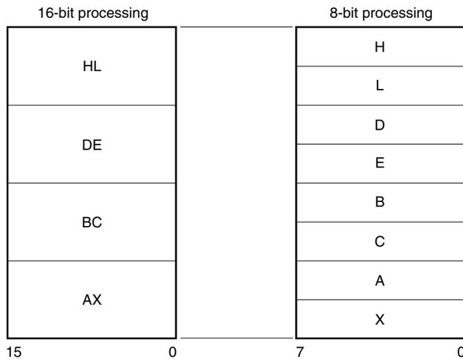
**Figure 3-12. General-Purpose Register Configuration (2/2)**
