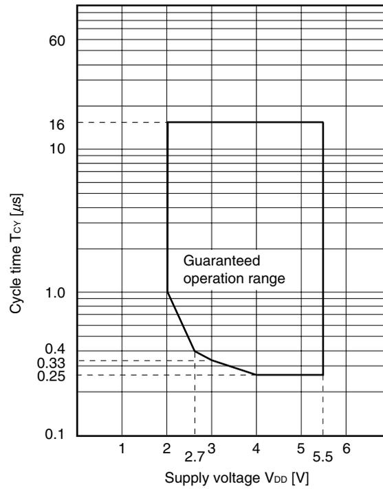
**$T_{CY}$  vs.  $V_{DD}$  (High-Speed Internal Oscillation Clock)**
