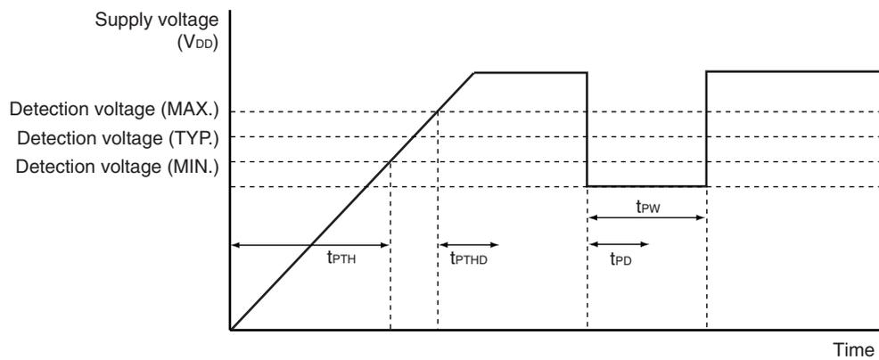
LVI Circuit Characteristics ( $T_A = -40$  to  $+85^\circ\text{C}$ )
