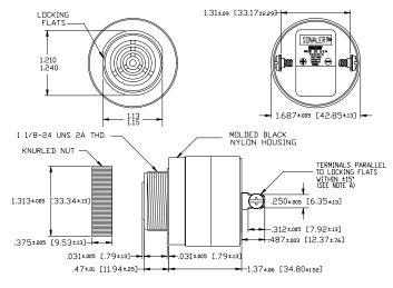
NOTE A: TERMINALS-032 BRASS TIN PLATED, TAPPED FOR #6-32 SCREW. TWO #6-32 NICKEL PLATED BRASS SCREWS INCLUDED. WILL ACCEPT 1/4\* QUICK CONNECT. NOTE B: MOUNTING- REMOVE BLACK PLASTIC NUT AND INSERT THREADED FRINT THROUGH 1.25' HOLE PUNCHED IN PANEL, IF DRIENTATION IS NEEDED, NOTE LOCKING FLATS ON DRAWING. SCREW NUT BACK ON. DO NOT OVERTIGHTEN.
