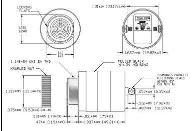
NOTE A: TERMINALS-032 BRASS TIN PLATED, TAPPED FOR #6-32 SCREW. TWO #6-32 NICKEL PLATED BRASS SCREWS INCLUDED. WILL ACCEPT 1/4' QUICK CONNECT. NOTE B: MOUNTING- REMOVE BLACK PLASTIC NUT AND INSERT THREADED FRONT THROUGH 125' HOLE PUNCHED IN PANEL, IF DRIENTATION IS NEEDED, NOTE LOCKING FLATS ON DRAVING, SCREW NUT BACK UN. DO NOT OVERTIGHTEN.
