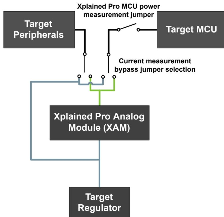
On the SAM L21 Xplained Pro the XAM can be used in four configurations:
