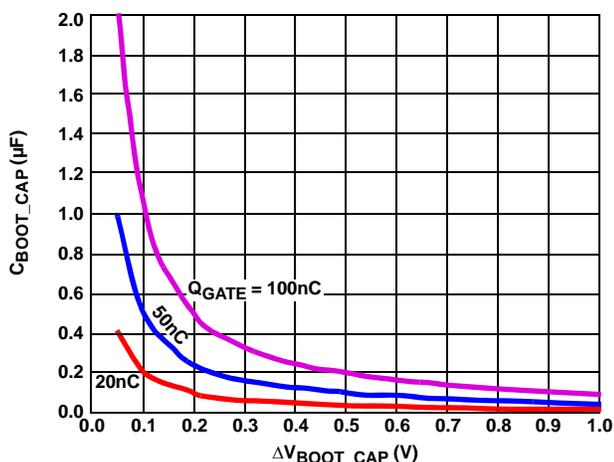
FIGURE 4. BOOTSTRAP CAPACITANCE vs BOOT RIPPLE VOLTAGE
