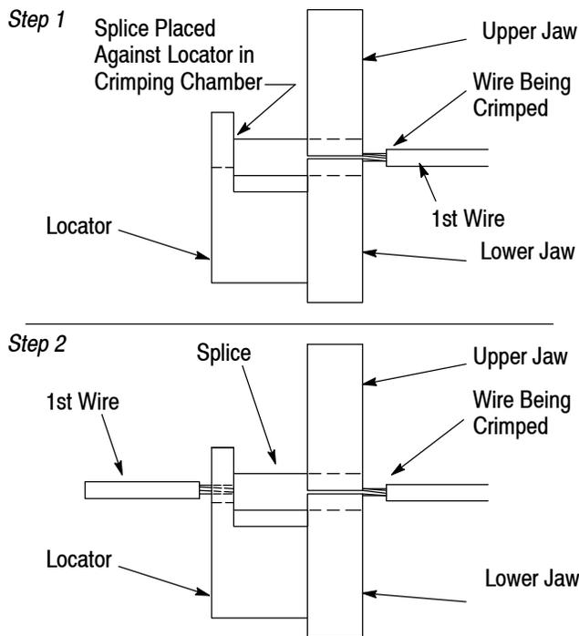
***If the wire is stripped correctly (Figure 2), the conductor will be exposed slightly more than the thickness of the locator. This will allow the conductor to enter the slot in the locator***
