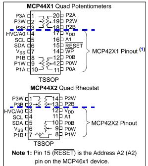
FIGURE 8-7: Quad Pinout (TSSOP Package) vs. Dual Pinout.
