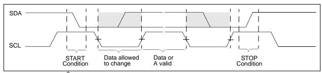
FIGURE 6-8: I<sup>2</sup>C Data States and Bit Sequence.
