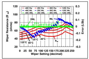
**FIGURE 2-17:** 10  $k\Omega$  Pot Mode –  $R_W$  ( $\Omega$ ), INL (LSb), DNL (LSb) vs. Wiper Setting and Ambient Temperature ( $V_{DD} = 5.5V$ ).
