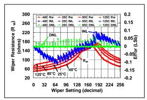
**FIGURE 2-40:** 100  $k\Omega$  Pot Mode –  $R_W$  ( $\Omega$ ), INL (LSb), DNL (LSb) vs. Wiper Setting and Ambient Temperature ( $V_{DD}$  = 3.0V).
