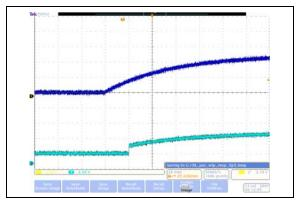
**FIGURE 2-14:**  $5 \text{ k}\Omega$  – Power-Up Wiper Response Time (20 ms/Div).
