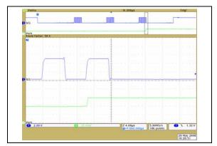
**FIGURE 2-27:** 10 k $\Omega$  – Low-Voltage Increment Wiper Settling Time ( $V_{DD}$  = 2.7V) (1  $\mu$ s/Div).
