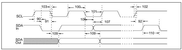
FIGURE 1-2: I<sup>2</sup>C Bus Data Timing.
