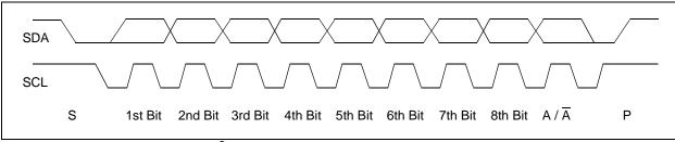
FIGURE 6-7: Typical 8-Bit I<sup>2</sup>C Waveform Format.
