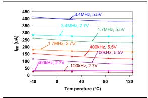
**FIGURE 2-1:** Device Current ( $I_{DD}$ ) vs.  ${}^{\hat{F}}C$  Frequency ( $f_{SCL}$ ) and Ambient Temperature ( $V_{DD} = 2.7V$  and 5.5V).
