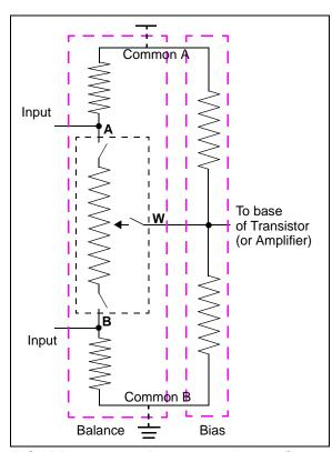
**FIGURE 8-1:** Example Application Circuit using Terminal Disconnects.
