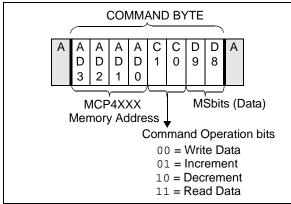
FIGURE 7-1: Command Byte Format.
