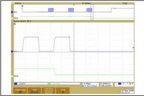
**FIGURE 2-35:** 50 kΩ – Low-Voltage Decrement Wiper Settling Time ( $V_{DD} = 2.7V$ ) (1 μs/Div).
