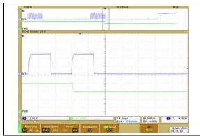
**FIGURE 2-12:**  $5 \text{ k}\Omega - \text{Low-Voltage}$  Decrement Wiper Settling Time ( $V_{DD} = 5.5V$ ) (1  $\mu$ s/Div).
