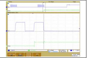
**FIGURE 2-47:** 100 kΩ – Low-Voltage Increment Wiper Settling Time ( $V_{DD}$ =5.5V) (1 μs/Div).
