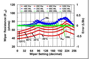
**FIGURE 2-19:** 10 kΩ Rheo Mode –  $R_W$  (Ω), INL (LSb), DNL (LSb) vs. Wiper Setting and Ambient Temperature ( $V_{DD}$  = 5.5V).
