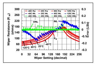
**FIGURE 2-18:** 10  $k\Omega$  Pot Mode –  $R_W$  ( $\Omega$ ), INL (LSb), DNL (LSb) vs. Wiper Setting and Ambient Temperature ( $V_{DD}$  = 3.0V).
