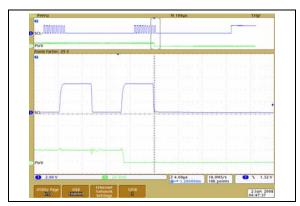
**FIGURE 2-46:** 100 kΩ – Low-Voltage Decrement Wiper Settling Time ( $V_{DD}$  = 2.7V) (1 μs/Div).
