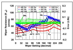
**FIGURE 2-6:** 5  $k\Omega$  Pot Mode –  $R_W$  ( $\Omega$ ), INL (LSb), DNL (LSb) vs. Wiper Setting and Ambient Temperature ( $V_{DD}$  = 5.5V).
