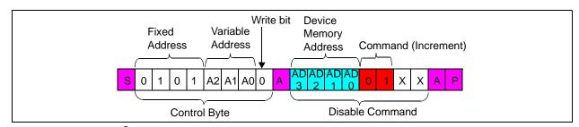
**FIGURE 7-9:** I<sup>2</sup>C Disable Command Sequence.
