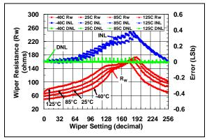
**FIGURE 2-42:** 100 kΩ Rheo Mode –  $R_W$  (Ω), INL (LSb), DNL (LSb) vs. Wiper Setting and Ambient Temperature ( $V_{DD}$  = 3.0V).
