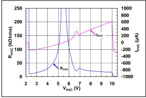
**FIGURE 2-4:** HVC Pull-up/Pull-down Resistance ( $R_{HVC}$ ) and Current ( $I_{HVC}$ ) vs. HVC Input Voltage ( $V_{HVC}$ ) ( $V_{DD} = 5.5V$ ).
