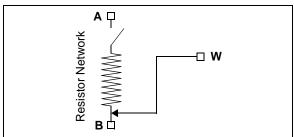
FIGURE 5-2: Resistor Network Shutdown Configuration.
