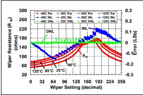
**FIGURE 2-29:** 50 kΩ Pot Mode –  $R_W$  (Ω), INL (LSb), DNL (LSb) vs. Wiper Setting and Ambient Temperature ( $V_{DD}$  = 3.0V).
