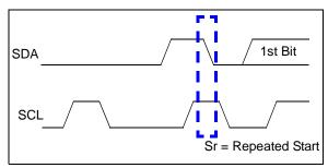
**FIGURE 6-5:** Repeat Start Condition Waveform.
