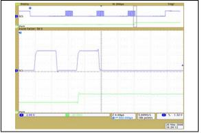
**FIGURE 2-26:** 10 k $\Omega$  – Low-Voltage Increment Wiper Settling Time ( $V_{DD} = 5.5V$ ) (1  $\mu$ s/Div).
