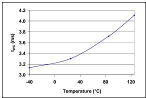
**FIGURE 2-56:** Nominal EEPROM Write Cycle Time vs. V<sub>DD</sub> and Temperature.
