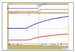
**FIGURE 2-36:** 50  $k\Omega$  – Power-Up Wiper Response Time (1  $\mu$ s/Div).
