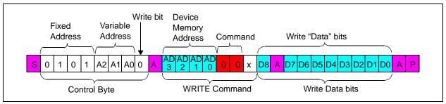
FIGURE 7-2: I<sup>2</sup>C Write Sequence.
