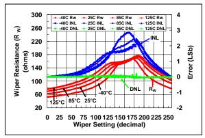
**FIGURE 2-20:** 10  $k\Omega$  Rheo Mode –  $R_W(\Omega)$ , INL (LSb), DNL (LSb) vs. Wiper Setting and Ambient Temperature ( $V_{DD} = 3.0V$ ).
