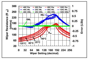
**FIGURE 2-31:** 50 k $\Omega$  Rheo Mode –  $R_W$  ( $\Omega$ ), INL (LSb), DNL (LSb) vs. Wiper Setting and Ambient Temperature ( $V_{DD}$  = 3.0V).
