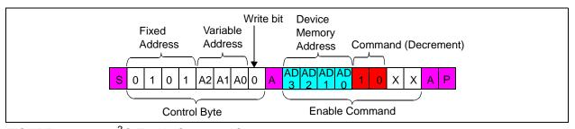
FIGURE 7-10: I<sup>2</sup>C Enable Command Sequence.
