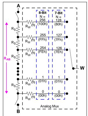
Note 1: The wiper resistance is dependent on several factors including, wiper code, device V<sub>DD</sub>, Terminal voltages (on A, B, and W), and temperature.
