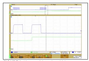
**FIGURE 2-16:**  $5 k\Omega - \text{Low-Voltage}$ Increment Wiper Settling Time ( $V_{DD} = 2.7V$ ) (1  $\mu$ s/Div).
