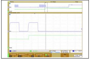
**FIGURE 2-15:**  $5 \text{ k}\Omega$  – Low-Voltage Increment Wiper Settling Time ( $V_{DD} = 5.5V$ ) (1  $\mu$ s/Div).
