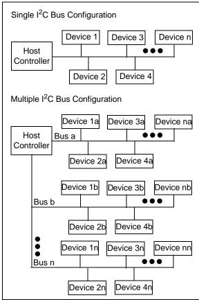
**FIGURE 8-3:** Typical Application I<sup>2</sup>C Bus Configurations.
