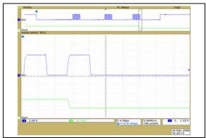
**FIGURE 2-24:** 10 kΩ – Low-Voltage Decrement Wiper Settling Time ( $V_{DD} = 2.7V$ ) (1 μs/Div).
