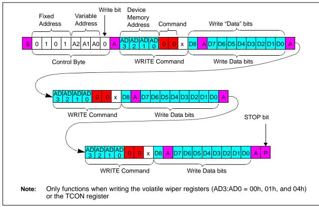
FIGURE 7-3: I<sup>2</sup>C Continuous Volatile Wiper Write.
