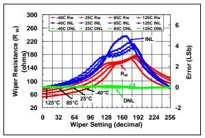
**FIGURE 2-9:** 5 kΩ Rheo Mode –  $R_W$  (Ω), INL (LSb), DNL (LSb) vs. Wiper Setting and Ambient Temperature ( $V_{DD}$  = 3.0V).
