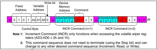
FIGURE 7-7: I<sup>2</sup>C Increment Command Sequence.
