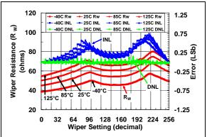
FIGURE 2-8: 5 kΩ Rheo Mode –  $R_W$  (Ω), INL (LSb), DNL (LSb) vs. Wiper Setting and Ambient Temperature ( $V_{DD}$  = 5.5V).
