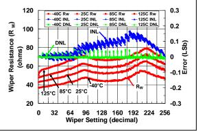
**FIGURE 2-41:** 100 kΩ Rheo Mode –  $R_W$  (Ω), INL (LSb), DNL (LSb) vs. Wiper Setting and Ambient Temperature ( $V_{DD}$  = 5.5V).
