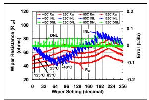
**FIGURE 2-39:** 100  $k\Omega$  Pot Mode –  $R_W$  ( $\Omega$ ), INL (LSb), DNL (LSb) vs. Wiper Setting and Ambient Temperature ( $V_{DD}$  = 5.5V).
