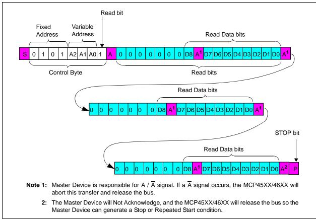
FIGURE 7-6: I<sup>2</sup>C Continuous Reads.
