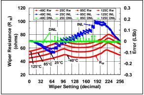
**FIGURE 2-30:** 50 kΩ Rheo Mode –  $R_W$  (Ω), INL (LSb), DNL (LSb) vs. Wiper Setting and Ambient Temperature ( $V_{DD}$  = 5.5V).
