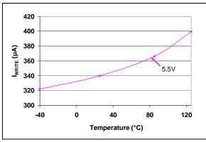
**FIGURE 2-3:** Write Current ( $I_{WRITE}$ ) vs. Ambient Temperature.
