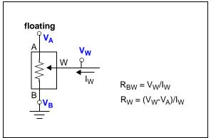
**FIGURE 2-59:**  $R_{BW}$  and  $R_{W}$  Measurement.
