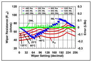
**FIGURE 2-28:** 50 k $\Omega$  Pot Mode –  $R_W$  ( $\Omega$ ), INL (LSb), DNL (LSb) vs. Wiper Setting and Ambient Temperature ( $V_{DD} = 5.5V$ ).
