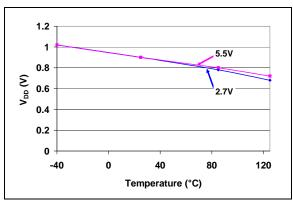
**FIGURE 2-57:** POR/BOR Trip Point vs.  $V_{DD}$  and Temperature.
