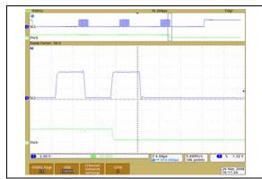
**FIGURE 2-34:** 50 kΩ – Low-Voltage Decrement Wiper Settling Time ( $V_{DD} = 5.5V$ ) (1 μs/Div).
