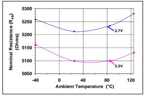
**FIGURE 2-10:** 5  $k\Omega$  – Nominal Resistance  $(\Omega)$  vs. Ambient Temperature and  $V_{DD}$ .
