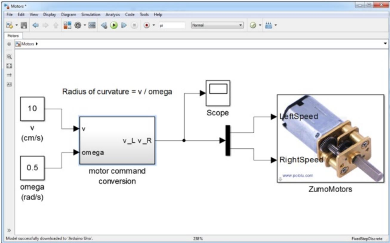
The model accepts velocity '**v**' and turning angle '**omega**' as inputs and using the subsystem named '**motor command conversion**' converts the two inputs into left and right wheel velocities.
