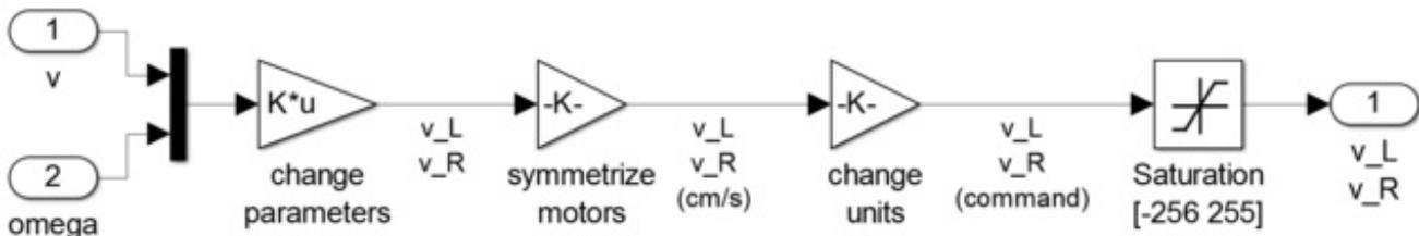
The first block named '**change parameters**' performs the matrix multiplication operation we saw in the equations above. To look at the block properties, double click on the block.
